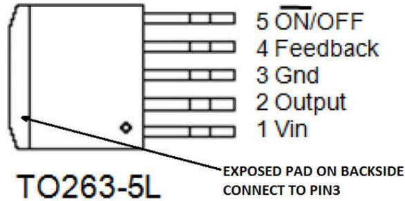
Figure 2. Pin Configuration of TD1602 (Top View)
