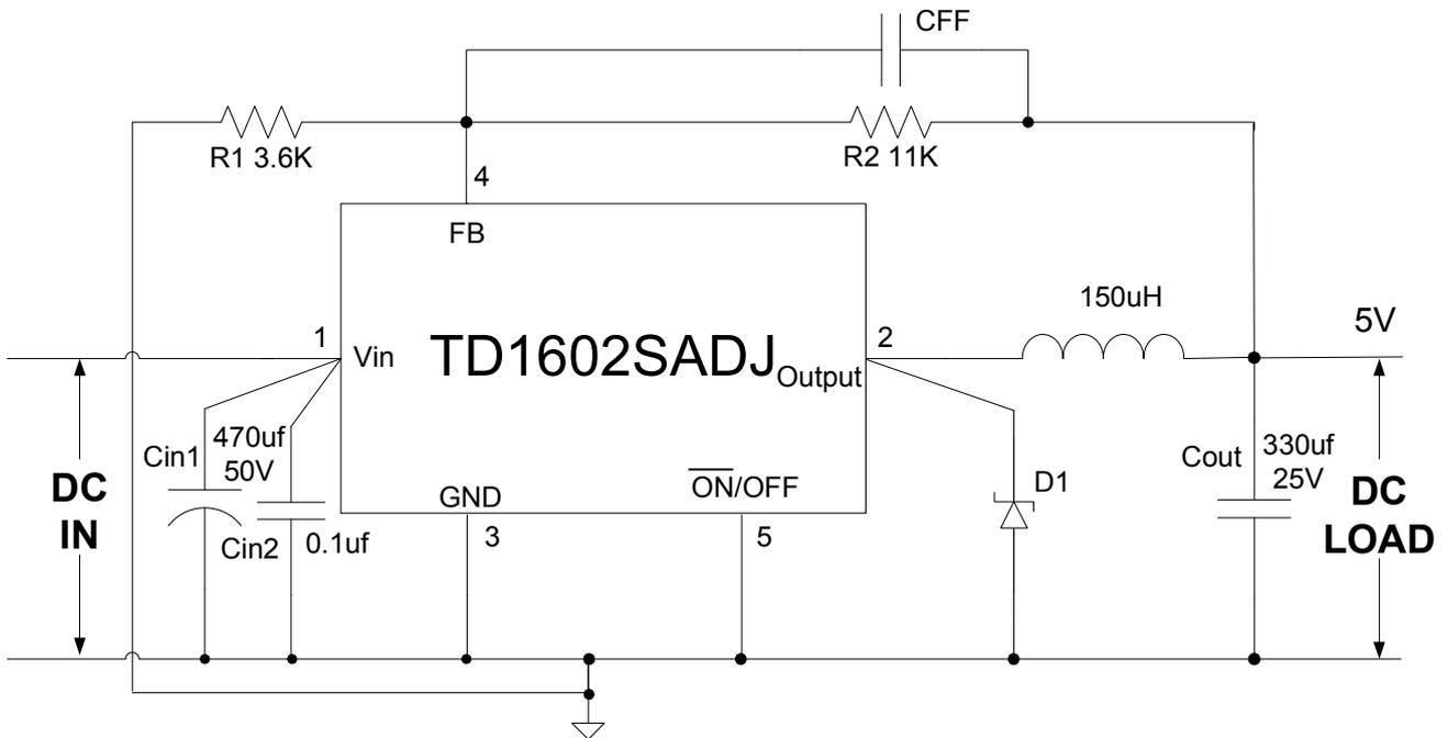
Figure 12. Typical Application of TD1602 For ADJ
