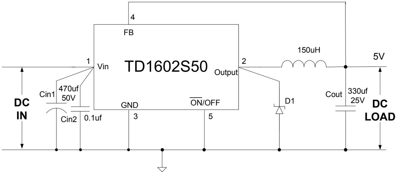
Figure 11. Typical Application of TD1602 For 5V
