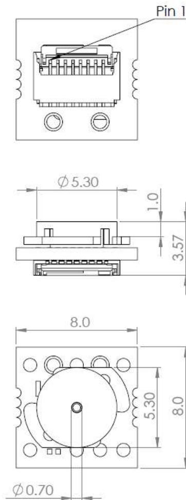
Figure 2. Main dimensions of the MOD\_CH101-03-01 assembly
