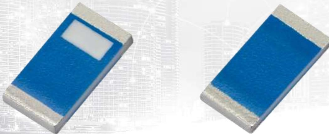
The WLA.10 2.4 / 5.8 GHz Loop antenna is a high efficiency, miniature SMD, edge mounted ceramic antenna for Dual-band 2.4 /5.8 GHz Wi-Fi and 802.11 applications where PCB space is limited, such as hand-held devices. The WLA.10 uses the main PCB as its ground plane, thereby maintaining good efficiency despite its small size. The efficiency is very stable on the complete bandwidth of both lower and upper bands allowing for maximum data throughput rates on all channels available.
