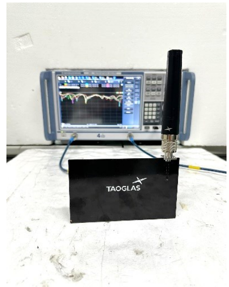
VNA Test Set-up – 15x9cm Ground Plane
