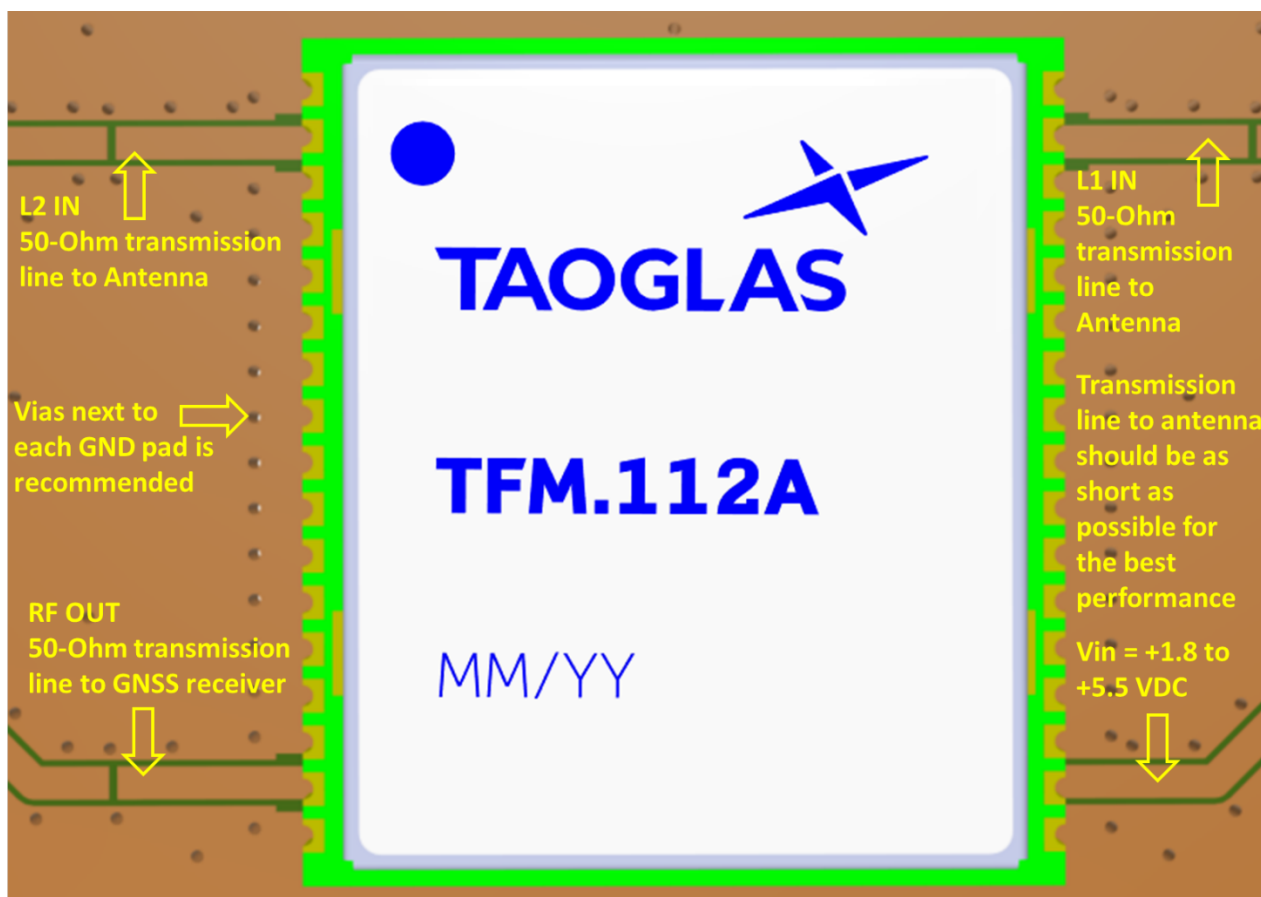
TFM.112A module mounted on a PCB, showing transmission lines and integration notes.
