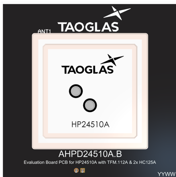
Top Side ( HP24510A placement on 70x70mm PCB)
