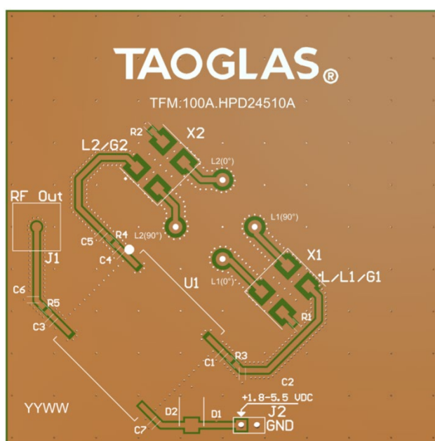
Top Side ( HP24510A placement on 70x70mm PCB)
