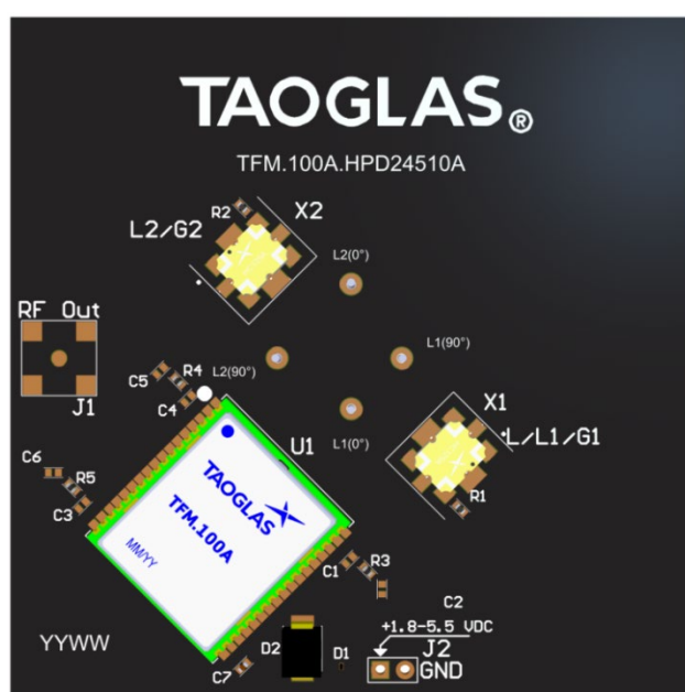
Top Side ( HP24510A placement on 70x70mm PCB)
