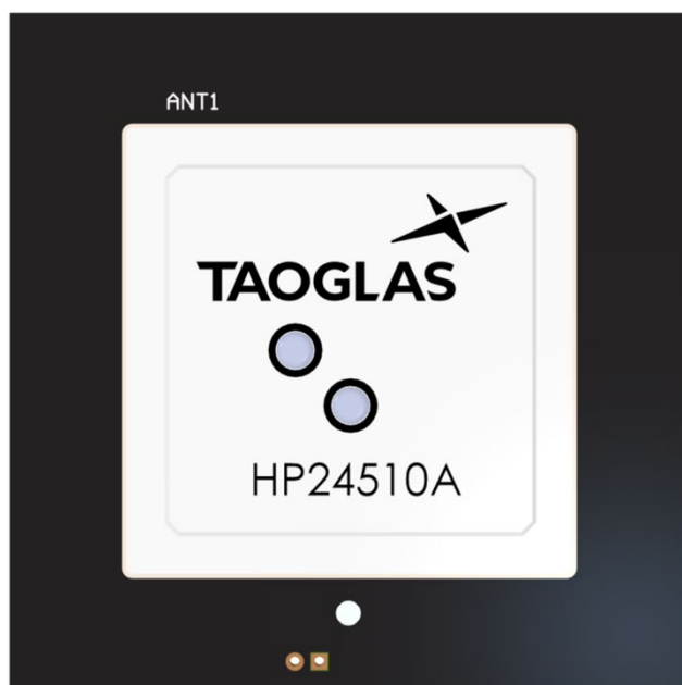
Top Side ( HP24510A placement on 70x70mm PCB)
