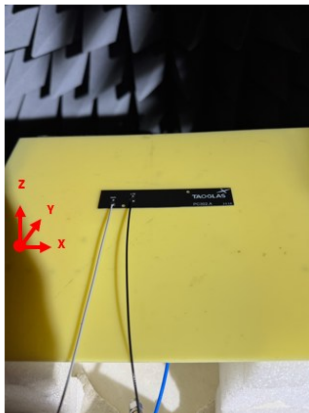
Chamber Test Setup on 2mm ABS
