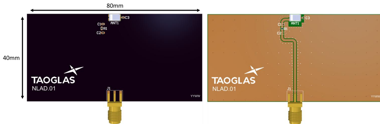
Top Side (NLAD.01 placement on 80x40mm PCB)
