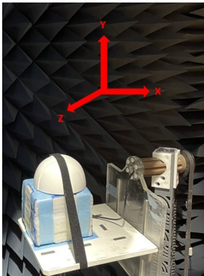
Chamber Test Set-up in Free Space
