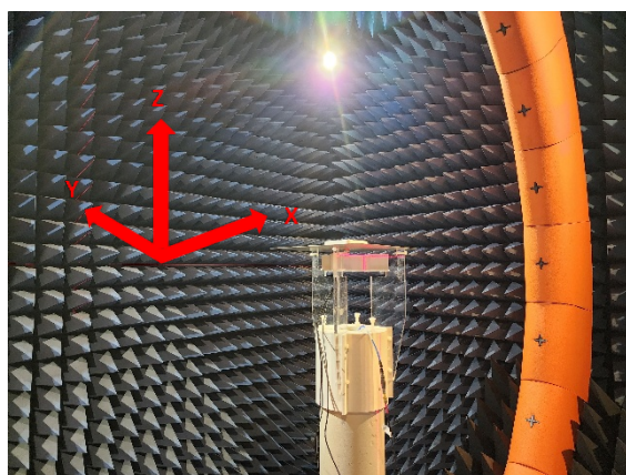
Set-up on a 30x30cm Ground Plane
