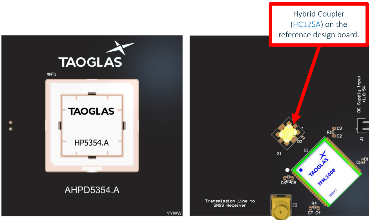
Above are the 3D models of the HP5354.A and HC125A on the reference design board.
