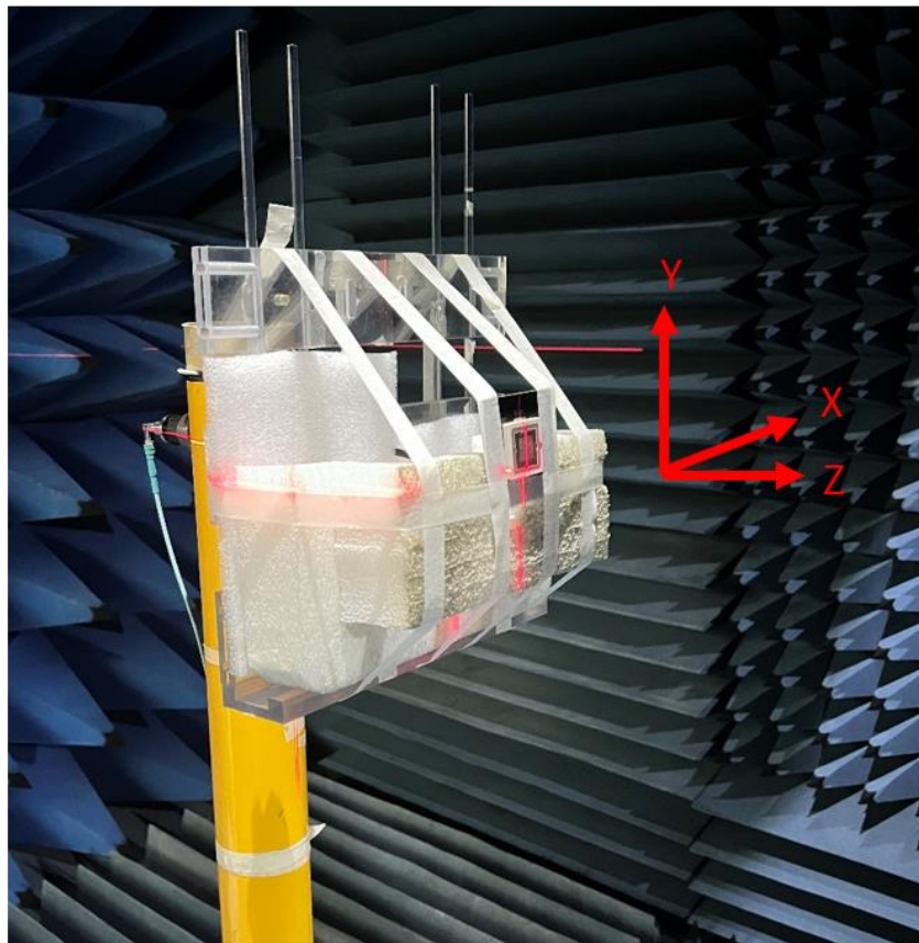
Chamber test setup on 70x70mm ground plane
