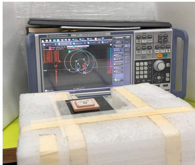
VNA Test Setup on 70x70mm Ground Plane
