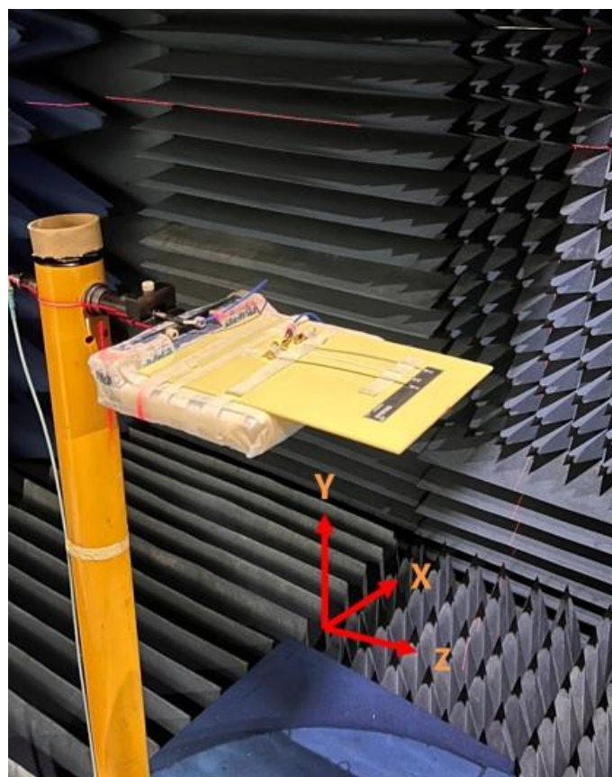
Chamber Test Setup on 2mm ABS
