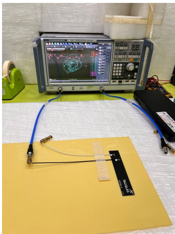
VNA Test Setup on 2mm ABS
