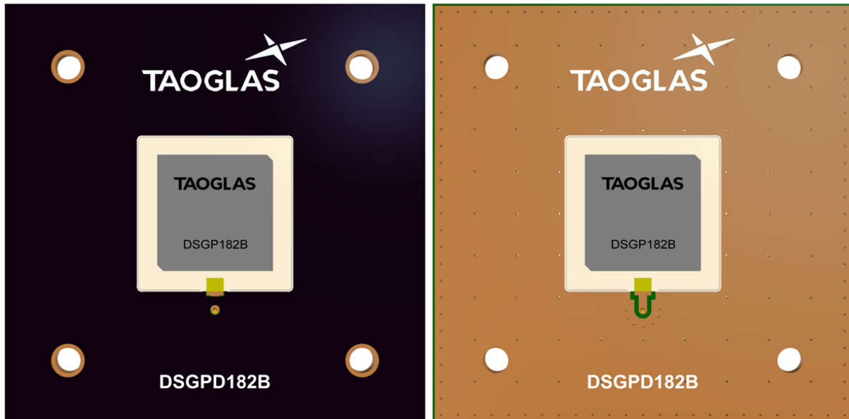
Top Side (DSGP182B placement on 50x50mm PCB reference design)
