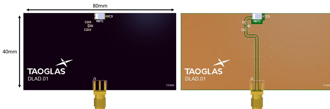
Top Side (DLA.01 placement on 80x40mm PCB)
