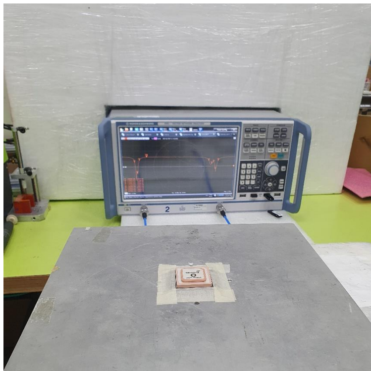
VNA Test Set-up on 30x30cm Metal Ground Plane
