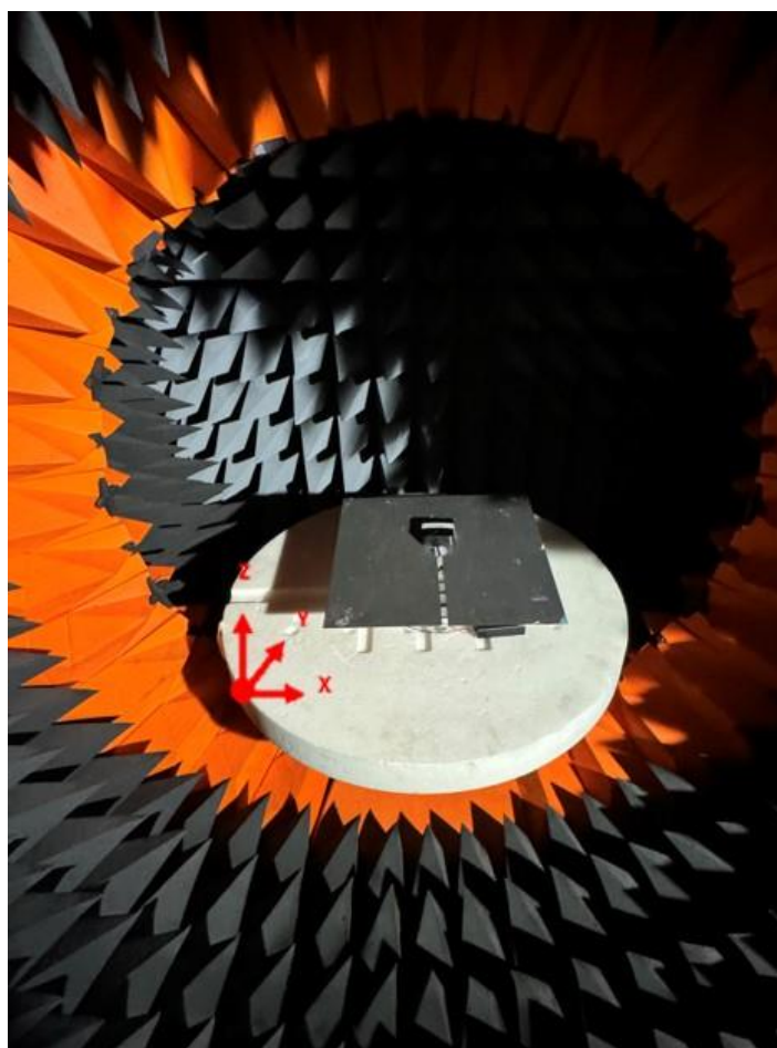
Test Set-up on a 30x30cm Metal Ground Plane
