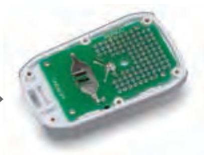
Install the PCB in the top cover
