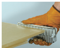
Work horizontally to collect dust
