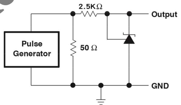
**Test Circuit for Pulse Response,  $I_{k} = 1\text{mA}$**
