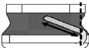
5. Electrode appearance criterion for exposed wire
