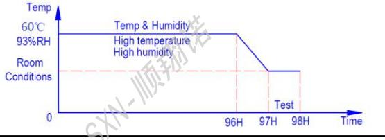
A graph showing temperature (Temp) in °C and humidity (93%RH) on the y-axis and time on the x-axis. The curve starts at Room Conditions, rises to a plateau labeled "Temp & Humidity" (60°C, 93%RH), remains constant for approximately 96 hours, then drops sharply to Room Conditions over about 1 hour, and finally levels off again. A vertical dashed line marks the start of the test at 96H. |
