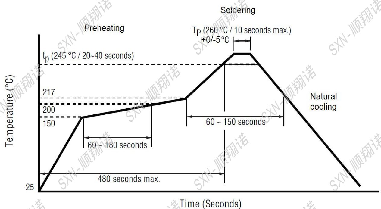
The recommended reflow conditions as above graph, is set according to our soldering equipment. DUE to various manufactures may have different reflow soldering equipment, products, process conditions, set methods. And so on, when setting the reflow conditions, Please adjust and confirm according to users' environment/equipment.
