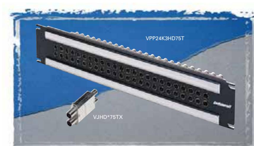
The VPP Series video patchbays offer a wide variety of options for video patching. The HD Series meets SMPTE 292M specifications for high definition video signaling, covering a bandwidth range from DC to 3.0GHz. The SD Series is perfect for serial digital, with a bandwidth from DC to 1.75GHz. Both come in either terminated or non-terminated, 24 or 26 jacks, 1.75" or 3.5" heights.
