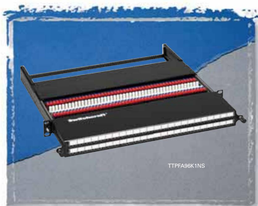
The Front Access Series offers the end user the ease of re-terminating patchpoints from the front of the rack as opposed to the back. A slide out tray allows the user to slide out the punchdown terminals and reconfigure the unit. An easy release mechanism on either side of the unit allows it to be pushed back into place and easy to grip locking nuts tighten the unit in place.
