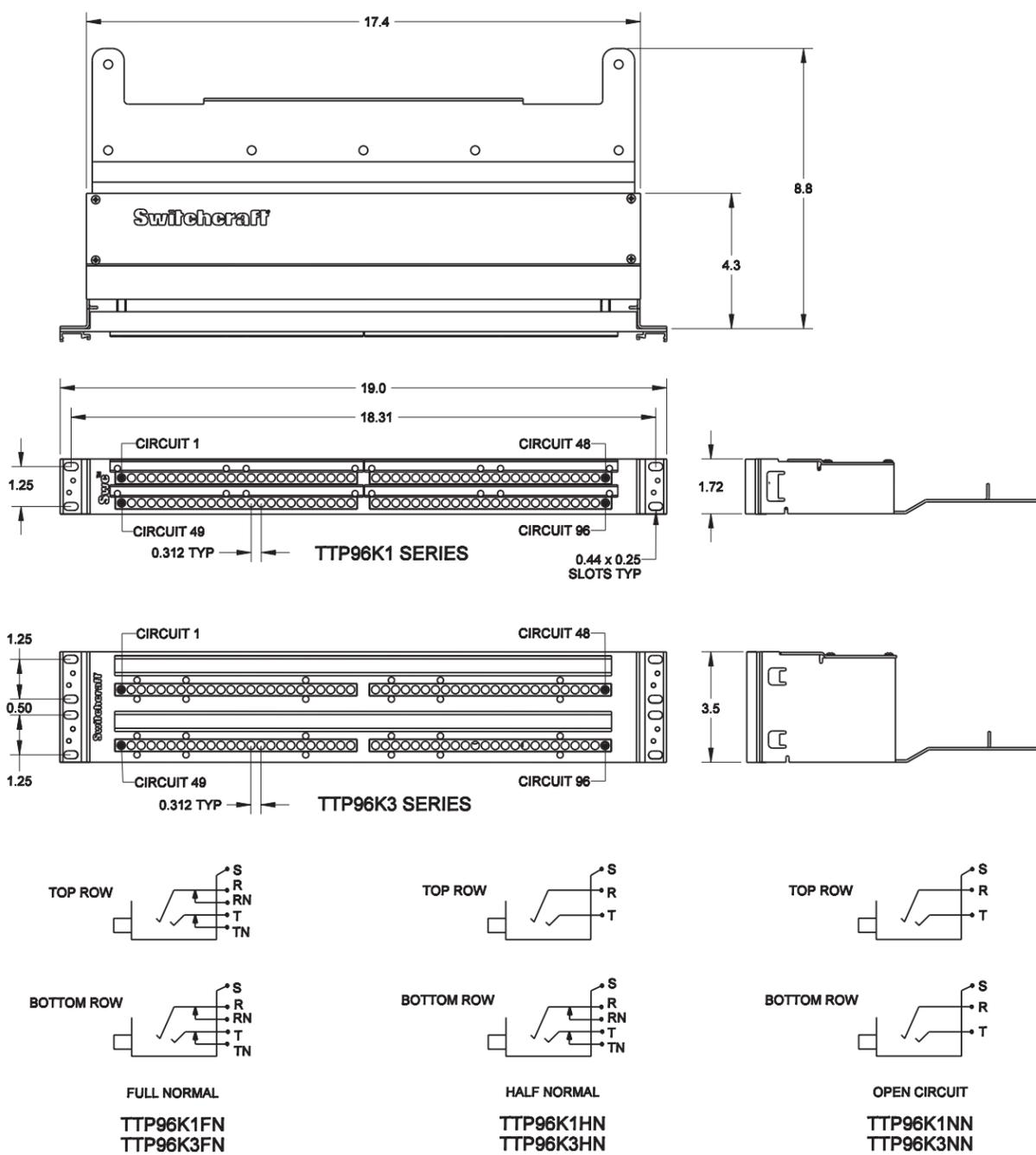
DIMENSIONS ARE FOR REFERENCE ONLY  $\frac{\text{Inch}}{\text{(mm)}}$
