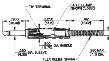
DIMENSIONS ARE FOR REFERENCE ONLY  $\frac{\text{Inch}}{\text{(mm)}}$
