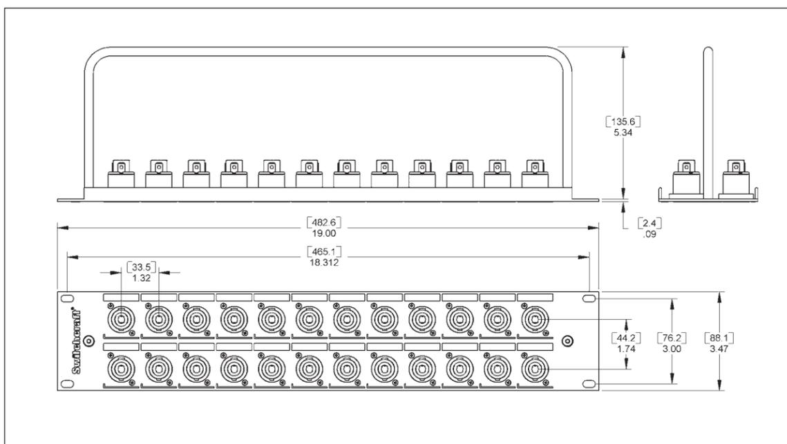
DIMENSIONS ARE FOR REFERENCE ONLY  $\frac{\text{Inch}}{\text{(mm)}}$
