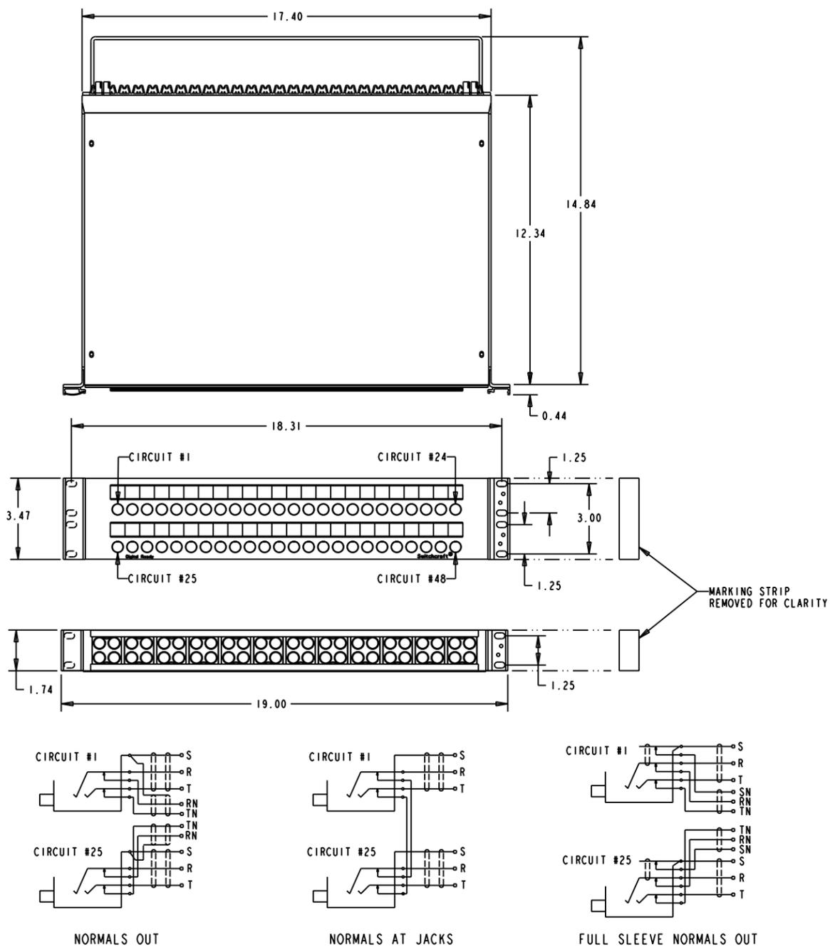
DIMENSIONS ARE FOR REFERENCE ONLY  $\frac{\text{Inch}}{\text{(mm)}}$
