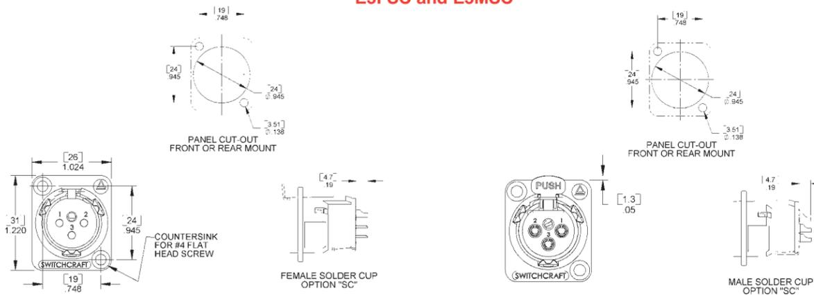
DIMENSIONS ARE FOR REFERENCE ONLY  $\frac{\text{Inch}}{\text{(mm)}}$
