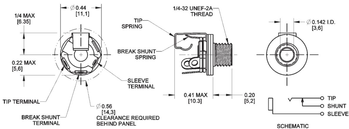
DIMENSIONS ARE FOR REFERENCE ONLY  $\frac{\text{Inch}}{\text{(mm)}}$
