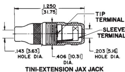
DIMENSIONS ARE FOR REFERENCE ONLY  $\frac{\text{Inch}}{\text{(mm)}}$
