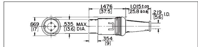
**Type 15GM7M – typical:** Male cord plug with shielded barrel and insulated snaplock plastic body. Two piece metal barrel surrounds pin insert to form an electrical shield. The entire insert assembly is held together by snapping the insulated plastic shell over the assembly. The barrel's special metal tab locks the shell in place. Standard color of plastic shell is gray. All-purpose cable clamp.
