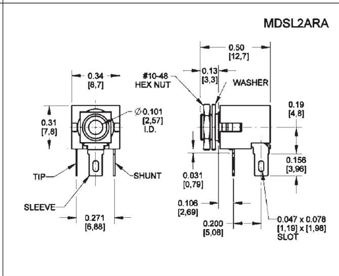
DIMENSIONS ARE FOR REFERENCE ONLY  $\frac{\text{Inch}}{\text{(mm)}}$
