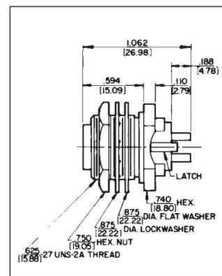
Rear of panel mount; 2 through 5 pins (male) or 2 through 5 contacts (female). Also 2-, 3- and 4-contact inserts with 2 shunted (N.C.) contacts. Mounting locknut (Part Number SL01), lock washer (Part Number SL02), and flat washer (Part Number SL03) supplied.
