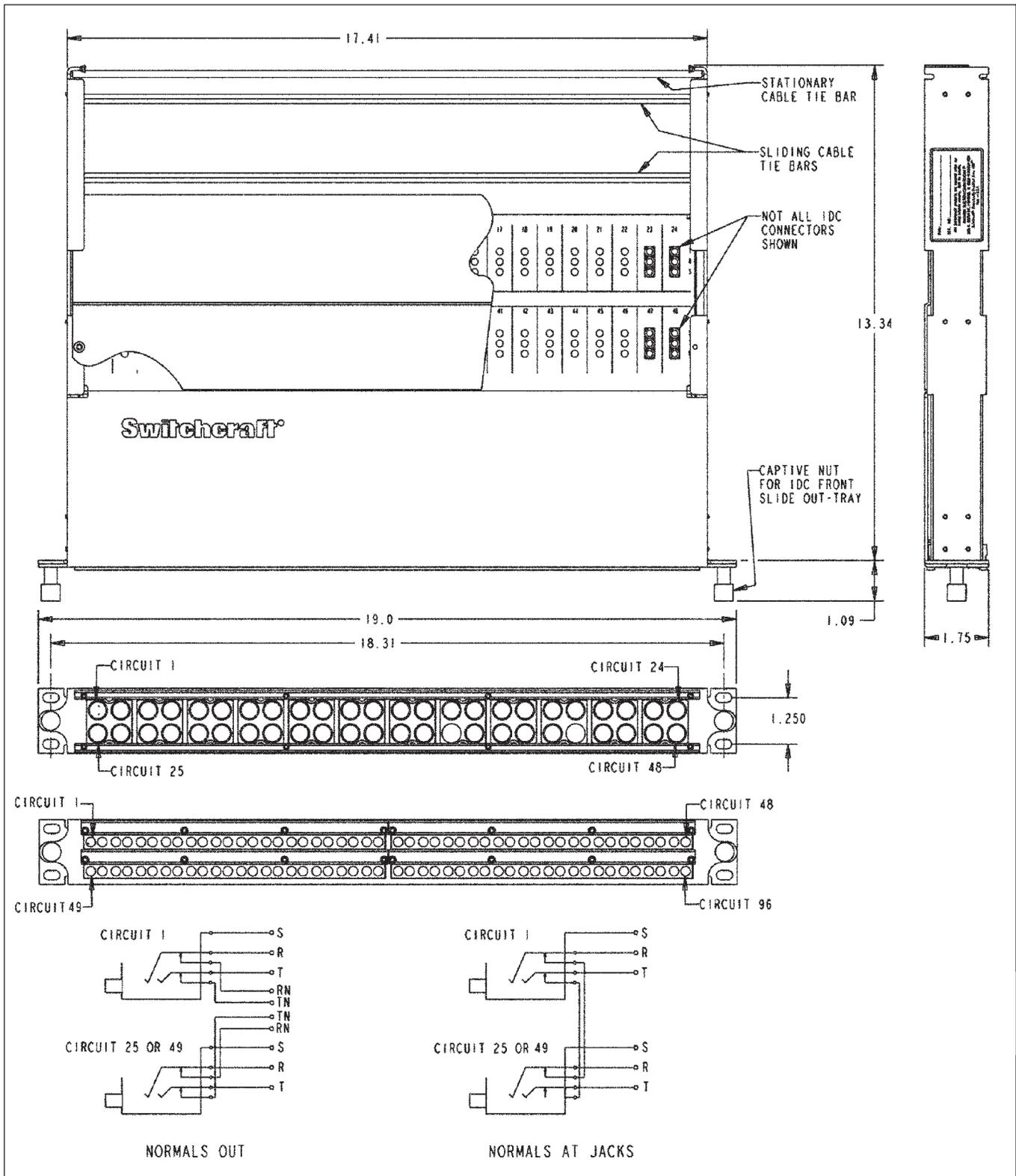
DIMENSIONS ARE FOR REFERENCE ONLY  $\frac{\text{Inch}}{(\text{mm})}$
