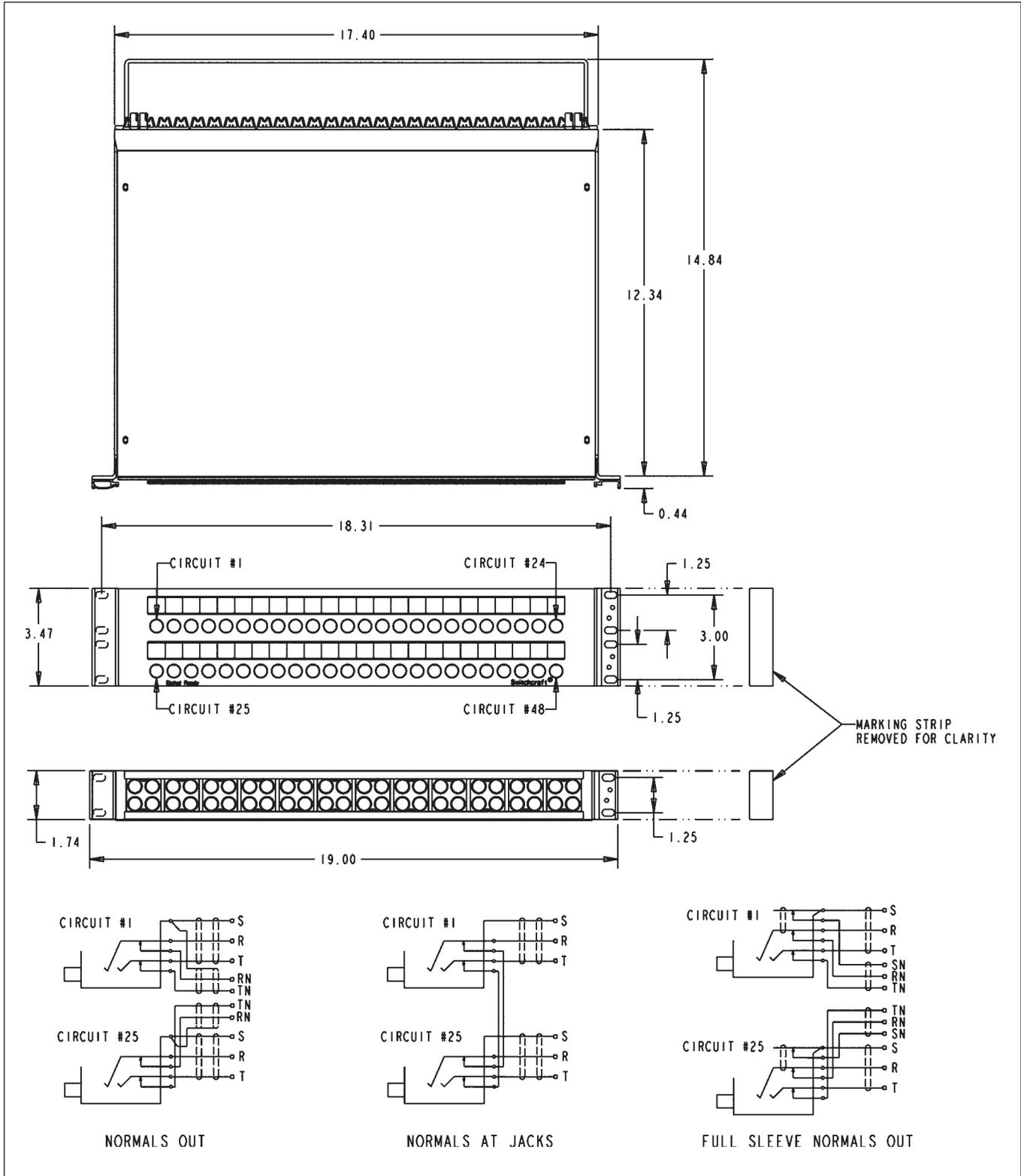
DIMENSIONS ARE FOR REFERENCE ONLY  $\frac{\text{Inch}}{(\text{mm})}$
