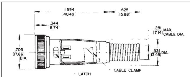
Non-reflective metal shell; coupling ring; 2 through 5 pins (male) or 2 through 5 contacts (female). Also 2-, 3- and 4-contact inserts with two shunted (N.C.) contacts. Efficient cable clamp and strain relief.
