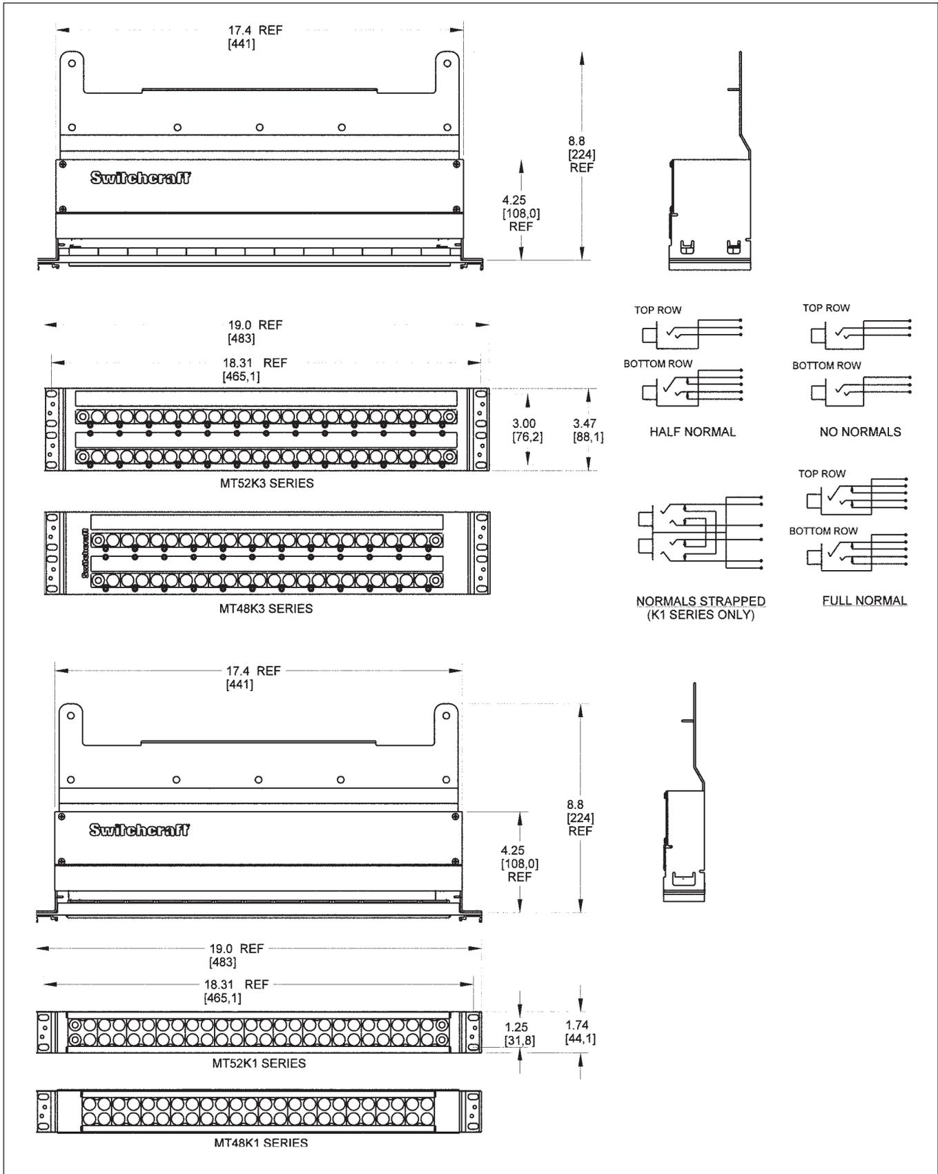
DIMENSIONS ARE FOR REFERENCE ONLY  $\frac{\text{Inch}}{\text{(mm)}}$
