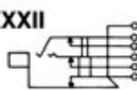
Double closed circuit. Separate sleeve "break" circuit.
