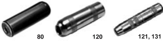
Extension Jax® jacks are connected to the end of a cable. 2- and 3-conductor jacks mate with standard commercial phone plugs, and have a sturdy cable clamp strain relief, knurled shielded or molded black plastic handles, and a screw type solder terminal. All internal parts are interlocked. Note: See locking phone plugs section.
