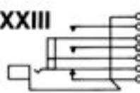
Single closed circuit. Isolated switching—Two "make" circuits.
