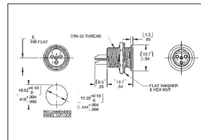
DIMENSIONS ARE FOR REFERENCE ONLY  $\frac{\text{Inch}}{\text{(mm)}}$
