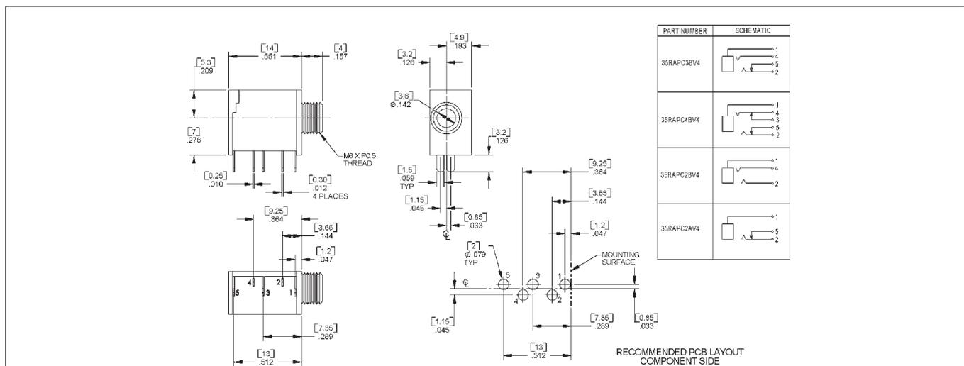
DIMENSIONS ARE FOR REFERENCE ONLY  $\frac{\text{Inch}}{(\text{mm})}$
