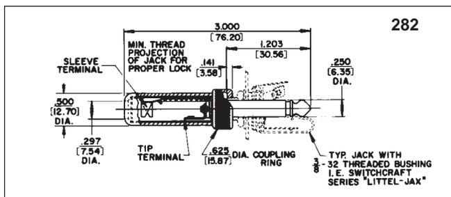
DIMENSIONS ARE FOR REFERENCE ONLY  $\frac{\text{Inch}}{(\text{mm})}$
