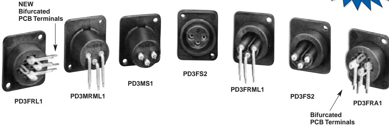
Switchcraft offers the PD Series (plastic panel mount) audio connectors with a wide variety of 3-pin/contact, male and female types and many terminals for combined PC/panel mount. Female types offer larger contact area for higher ratings and longer life. Panel mounting may be at users option, either front or rear. New PD series connectors mate with Switchcraft Q-G and other compatible types.
