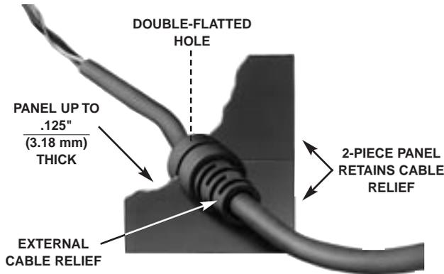
CUTAWAY VIEW OF STYLE ST303
