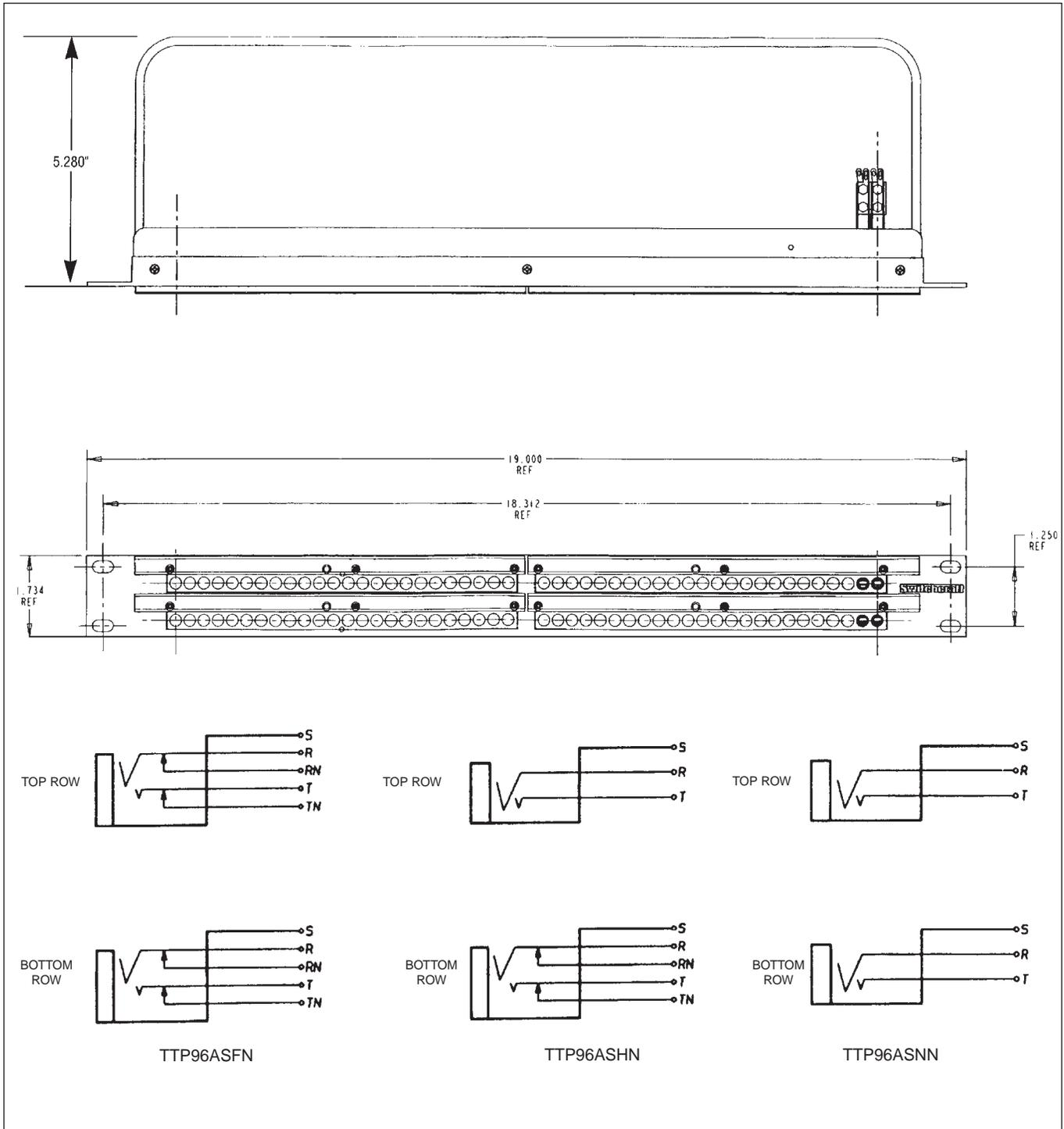
DIMENSIONS ARE FOR REFERENCE ONLY  $\frac{\text{Inch}}{\text{(mm)}}$
