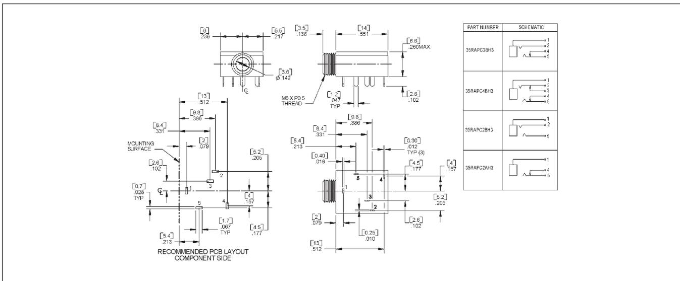
DIMENSIONS ARE FOR REFERENCE ONLY  $\frac{\text{Inch}}{\text{(mm)}}$
