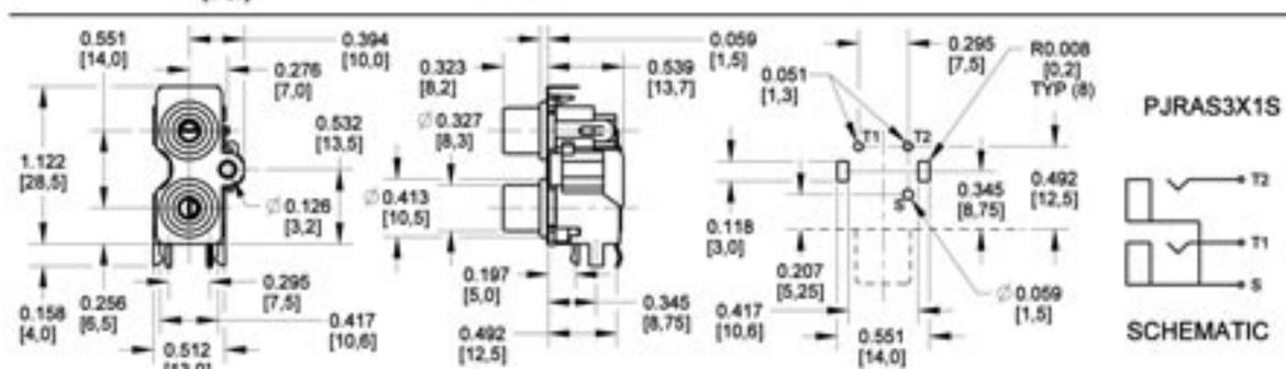
DIMENSIONS ARE FOR REFERENCE ONLY  $\frac{\text{Inch}}{\text{(mm)}}$
