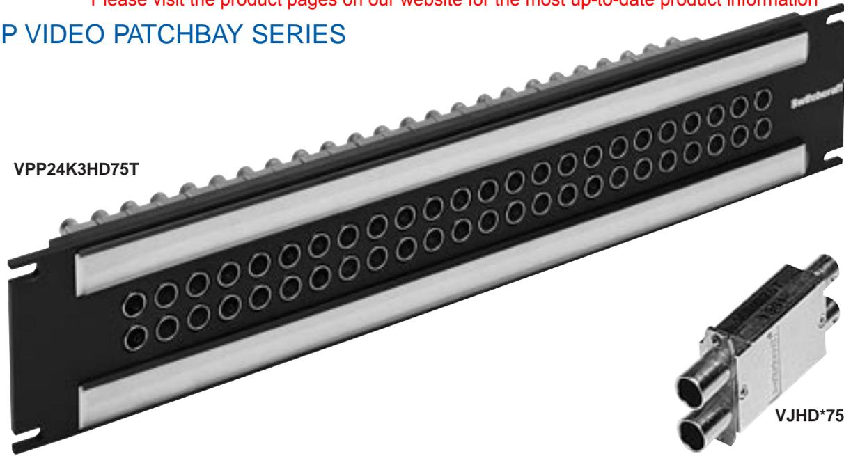
The VPP Series video patchbays offer a wide variety of options for video patching. The HD Series meets SMPTE 292M specifications for high definition video signaling, covering a bandwidth range from DC to 2.4GHz. The SD Series is perfect for serial digital, with a bandwidth from DC to 1.75GHz. Both come in either terminated or non-terminated, 24 or 26 jacks, 1.75" or 3.5" heights.
