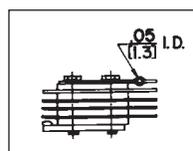
**Bus type terminals which allow you to buss jacks quickly and easily are available on special order.**
