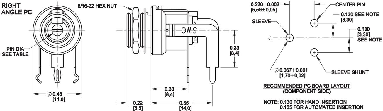
NOTE: "D" HOLE FLAT IS ON THE BOTTOM OF RIGHT ANGLE JACKS
