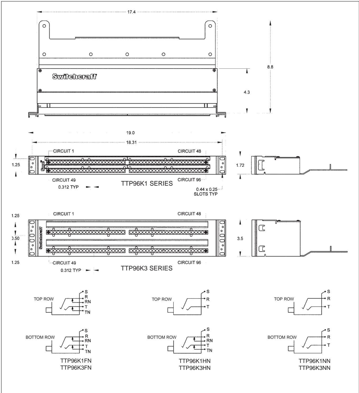
DIMENSIONS ARE FOR REFERENCE ONLY  $\frac{\text{Inch}}{\text{(mm)}}$
