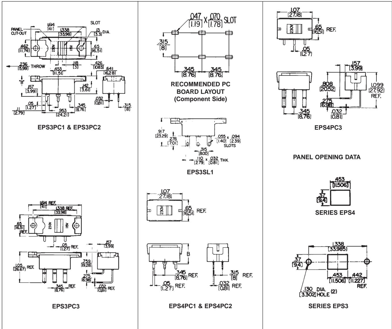
DIMENSIONS ARE FOR REFERENCE ONLY  $\frac{\text{Inch}}{\text{(mm)}}$
