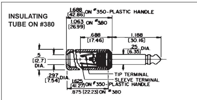
DIMENSIONS ARE FOR REFERENCE ONLY  $\frac{\text{Inch}}{\text{(mm)}}$
