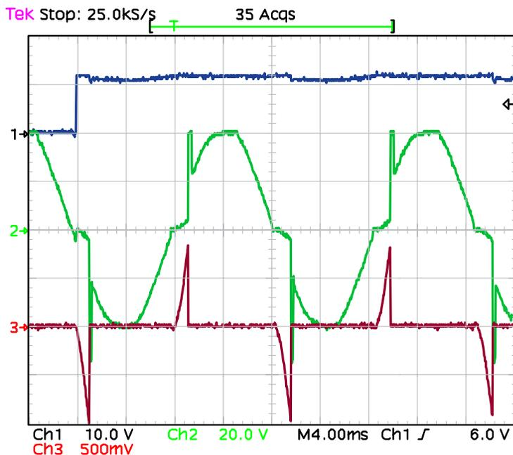
Enable from low to high into a shorted solenoid.
