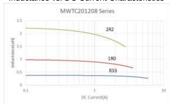
Inductance vs. DC Current Characteristics
