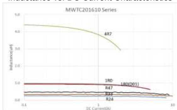
Inductance vs. DC Current Characteristics
