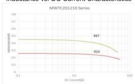
Inductance vs. DC Current Characteristics
