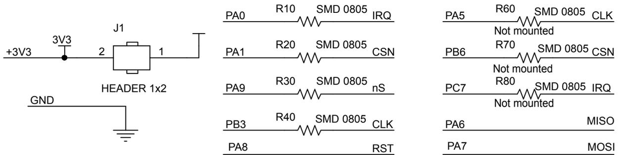
**Figure 3. X-NUCLEO-IDB05A2 circuit schematic - BlueNRG-M0A module**
