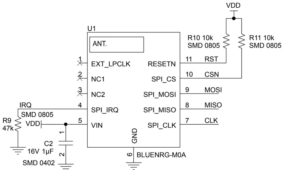
Figure 4. X-NUCLEO-IDB05A2 circuit schematic - EEPROM
