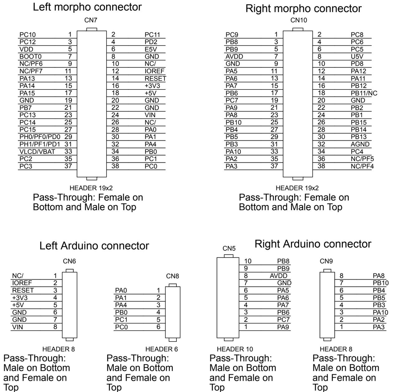
**Figure 2. X-NUCLEO-IDB05A2 circuit schematic - STM32 Nucleo connections**
