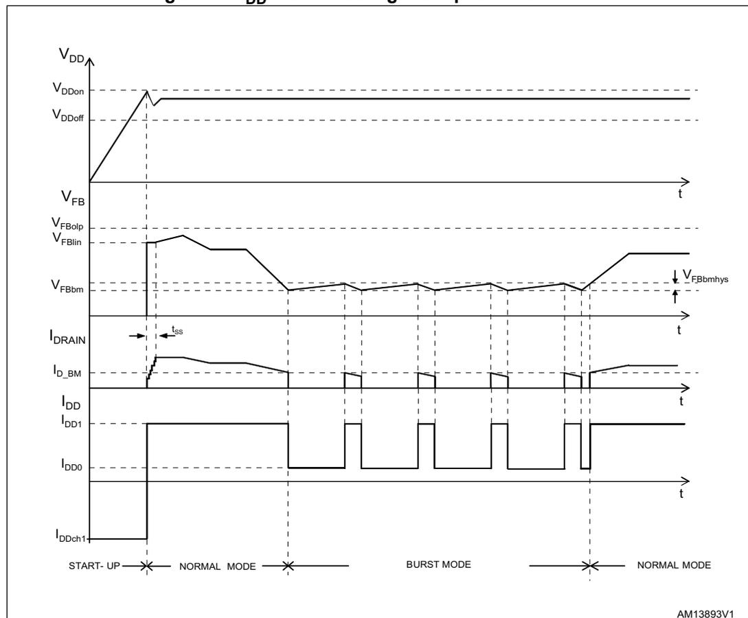
Figure 18. Timing diagram: normal power-up and power-down sequences
