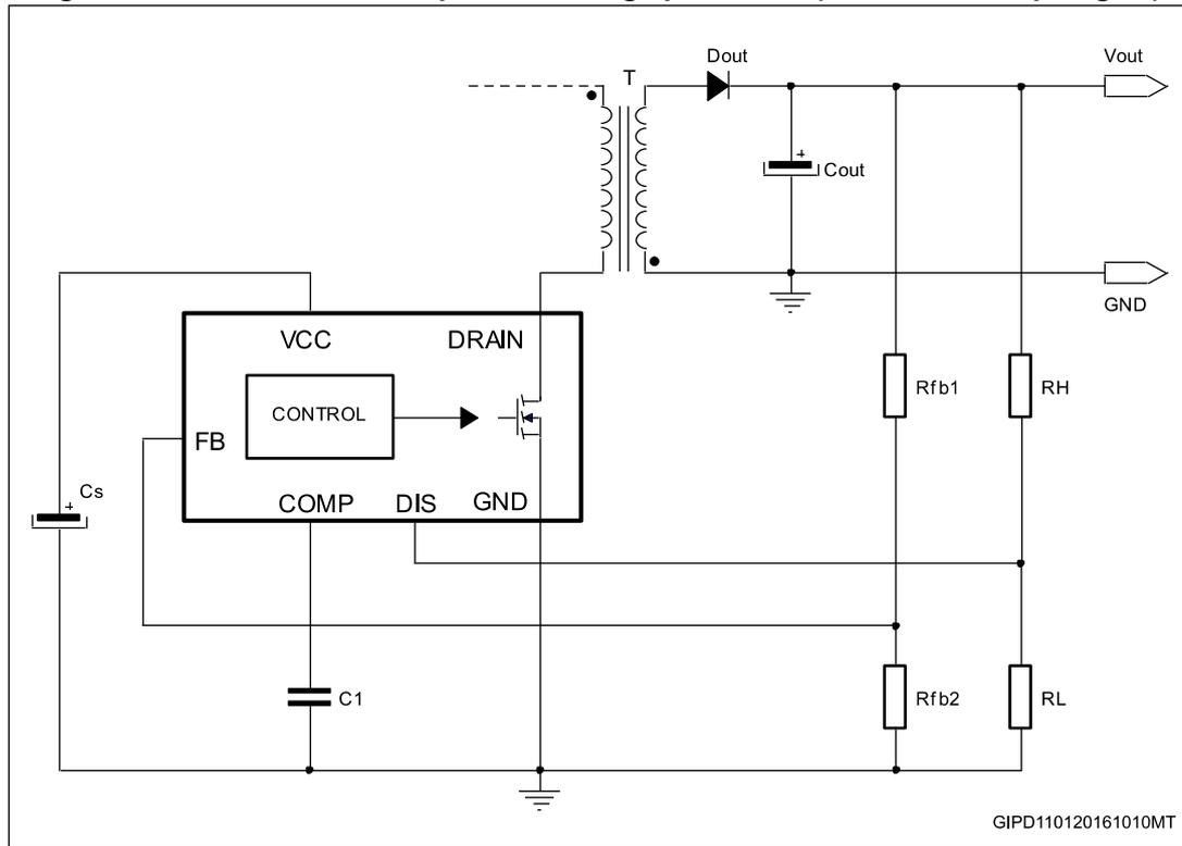
If  $V_{OVP}$  is the desired input/output overvoltage threshold, the resistors  $R_H$  and  $R_L$  of the voltage divider are to be selected according to the following formula:
