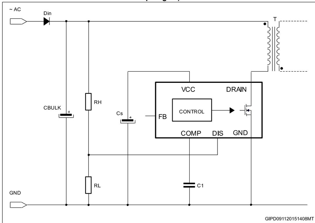
In case of non-isolated topologies, with the same principle an output overvoltage protection can be implemented, as shown in [Figure 32](#).
