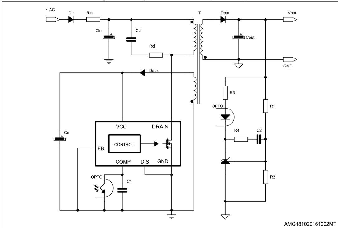
Figure 38. Primary side regulation isolated flyback converter
