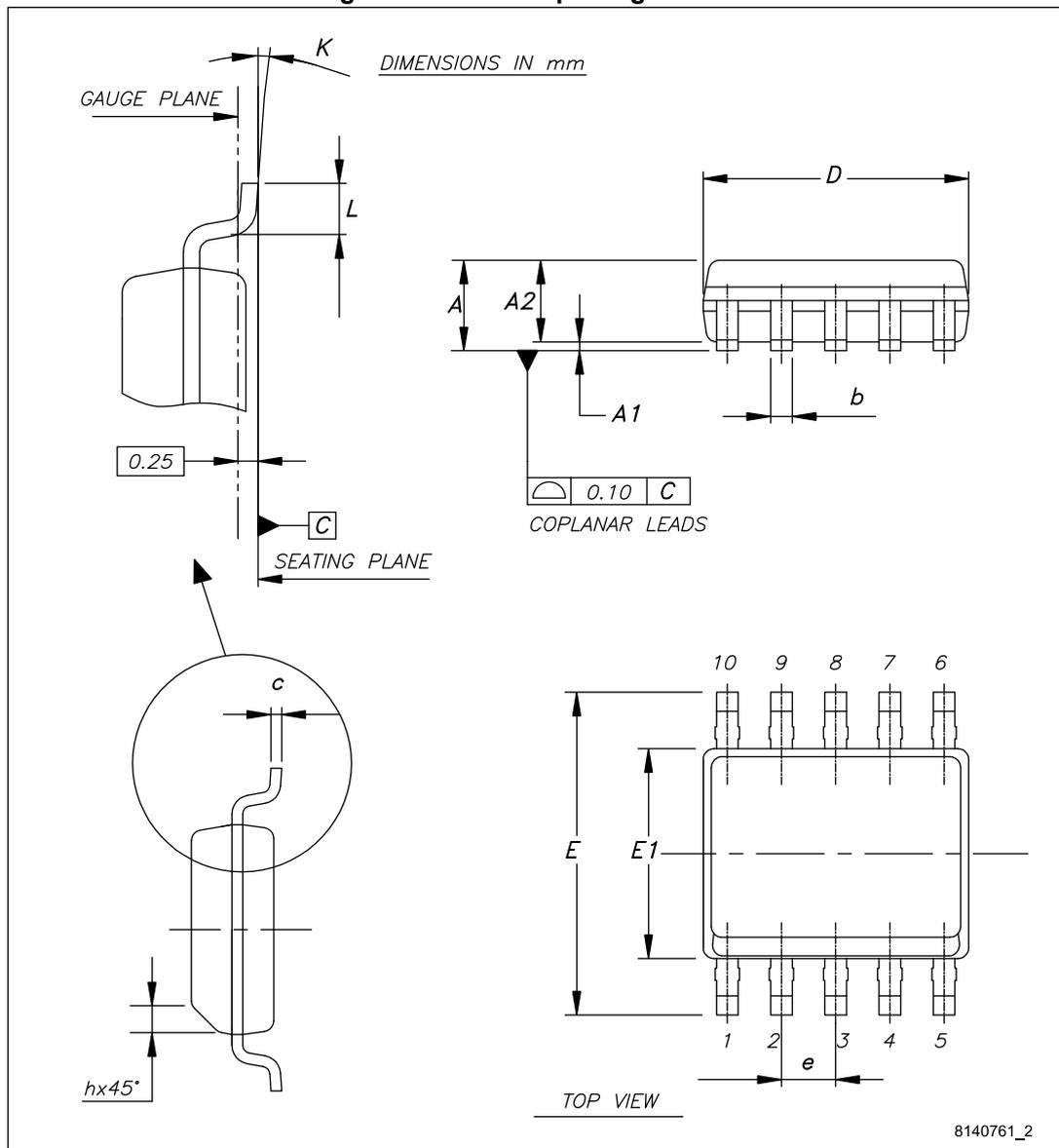
**Table 10. SSOP10 package mechanical data**
