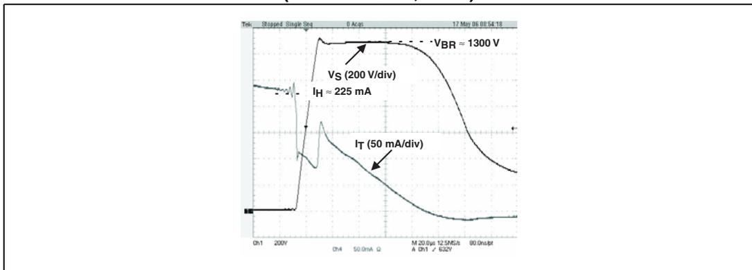
If the lamp is not ignited after the first pulse, the starter circuit starts a new ignition sequence. The pulse is regenerated until ignition of the tube lamp. If the lamp is not ignited after several attempts, the starter circuit can automatically stop the ignition sequence.
