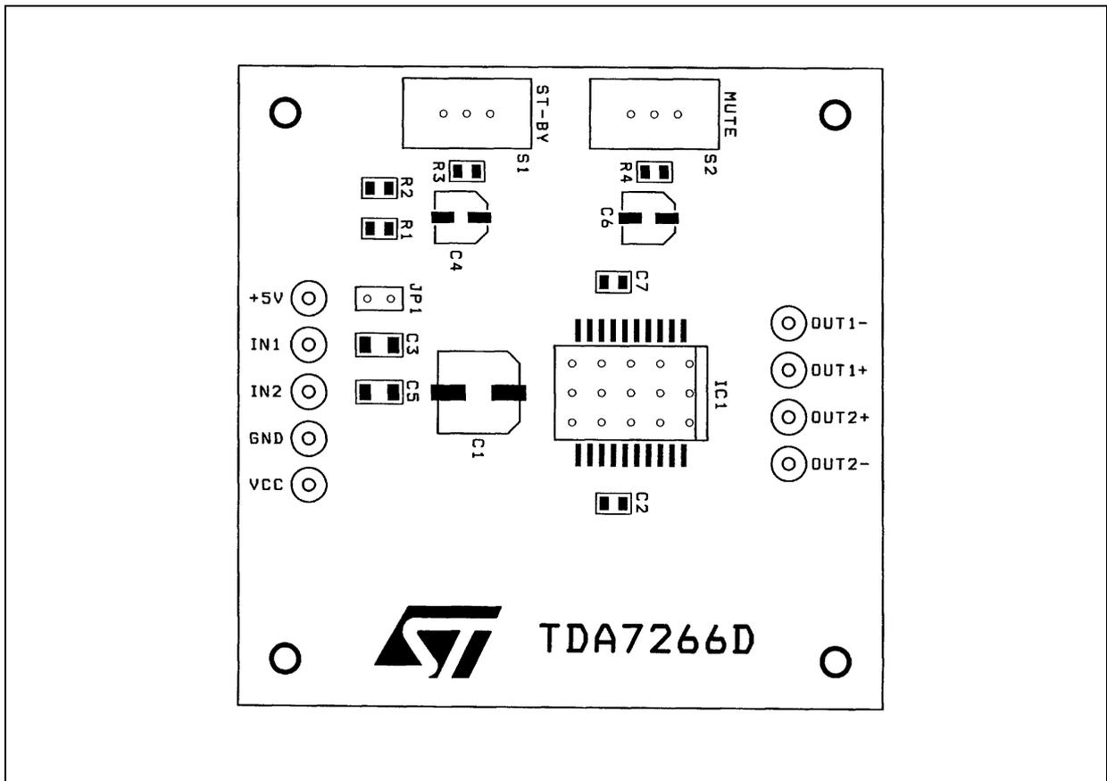
Figure 15. Evaluation Board Top Layer Layout
