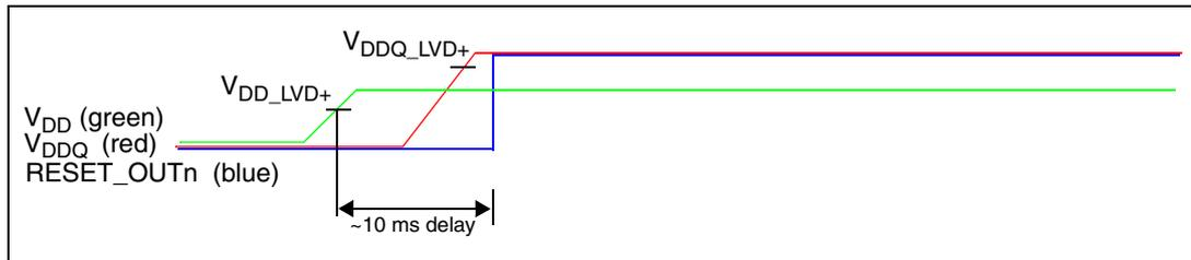
**Case 3:** When  $V_{DD}$  reaches the  $V_{DD\_LVD+}$  threshold **after** the  $V_{DDQ}$  rising edge, RESET\_OUTn will be released at the end of a  $\sim 10$  ms delay. See [Figure 14](#).
