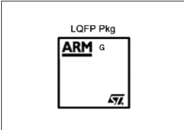
Figure 35. Device marking for revision G
