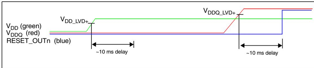
**Case 2:** When  $V_{DDQ}$  reaches the  $V_{DDQ\_LVD+}$  threshold **before** the first  $\sim 10$  ms delay (introduced by the VDD rising edge), RESET\_OUTn will be released immediately at the end of the delay. No new delay is introduced in this case. See [Figure 13](#).
