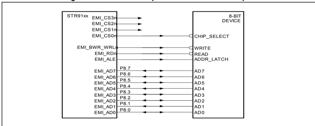
Figure 6. EMI 8-bit non-multiplexed connection example
