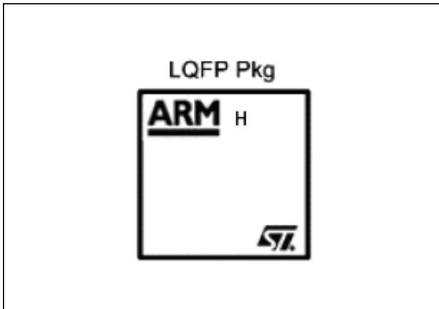
Figure 37. Device marking for revision H
