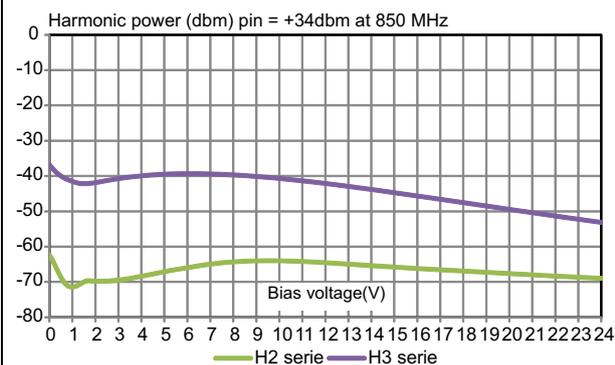
**Figure 5. Harmonic power versus bias voltage (shunt)**
