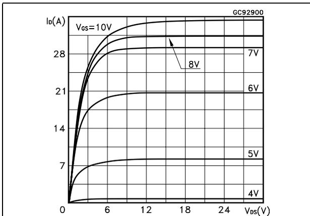
Figure 6. Transfer characteristics
