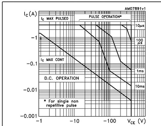
Figure 3. Derating curve
