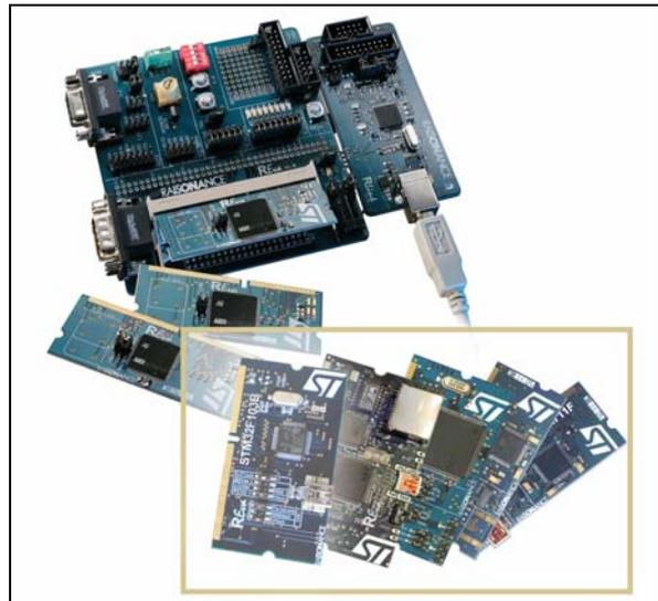
REva evaluation board, microcontrollers, embedded RLink JTAG in-circuit debugger/programmer and Raisonance Integrated Development Environment (RIDE).
