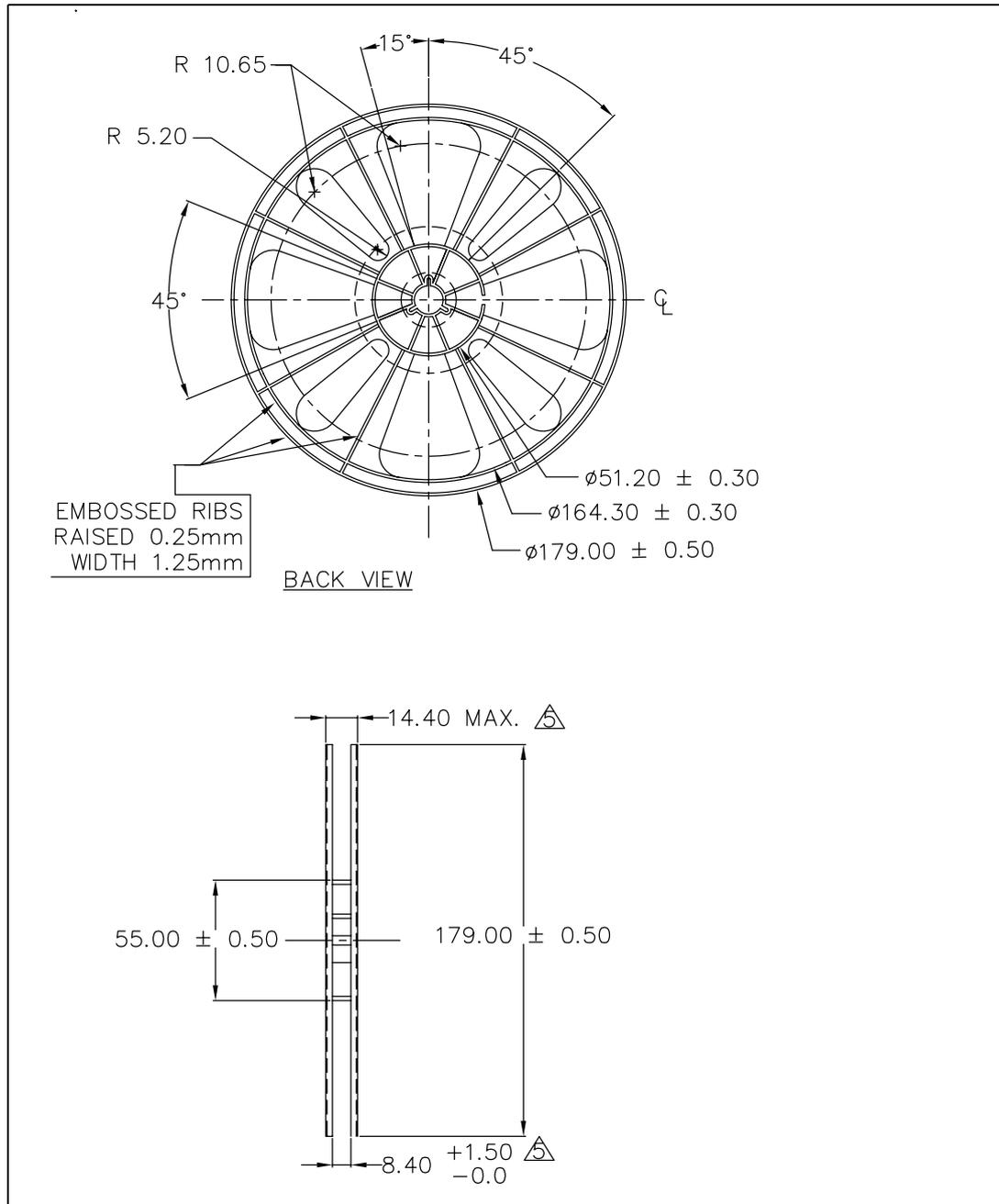
Figure 7. QFN12L (2.2 x 1.4 mm) reel for carrier tape information
