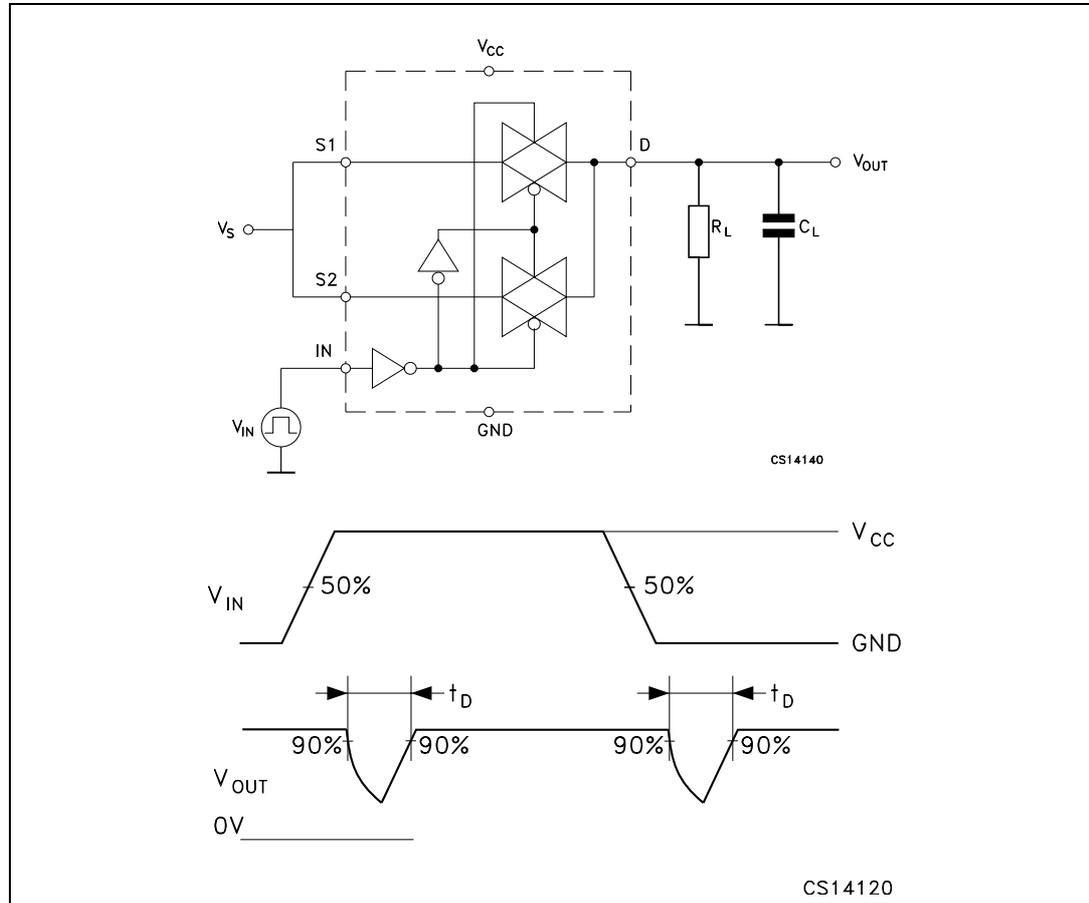
**Figure 10. Switching time and charge injection** ( $V_{GEN} = 0\text{ V}$ ,  $R_{GEN} = 0\ \Omega$ ,  $R_L = 1\text{ M}\Omega$ ,  $C_L = 100\text{ pF}$ )
