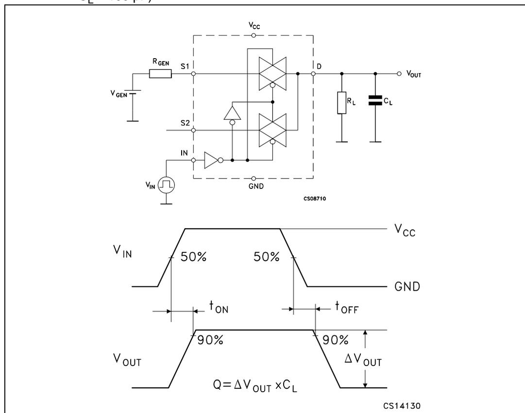
Figure 11. Turn ON, Turn OFF delay time
