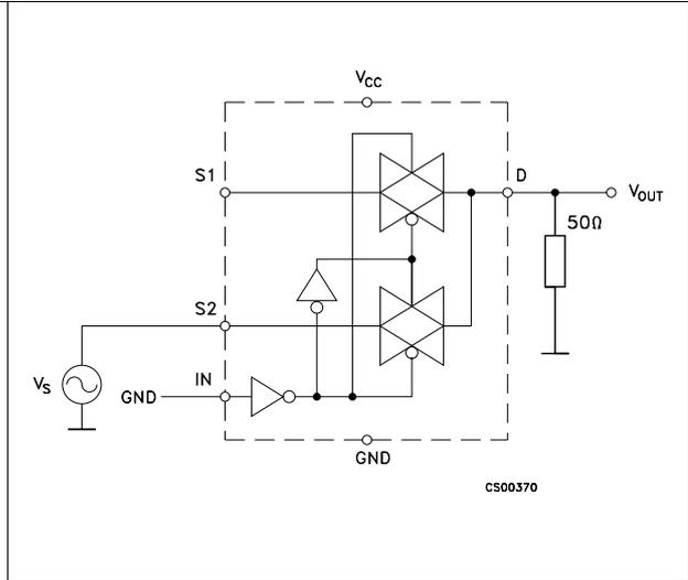
**Figure 5. OFF leakage**
