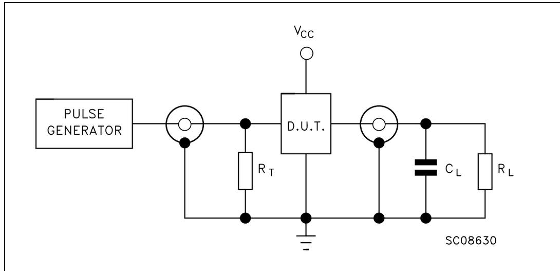
$C_L = 5/35$  pF or equivalent (includes jig and probe capacitance)
