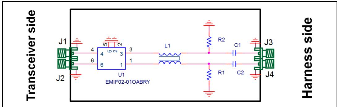
The board schematic shows four RF SMA connectors (J1, J2, J3 and J4) for the following connections:
