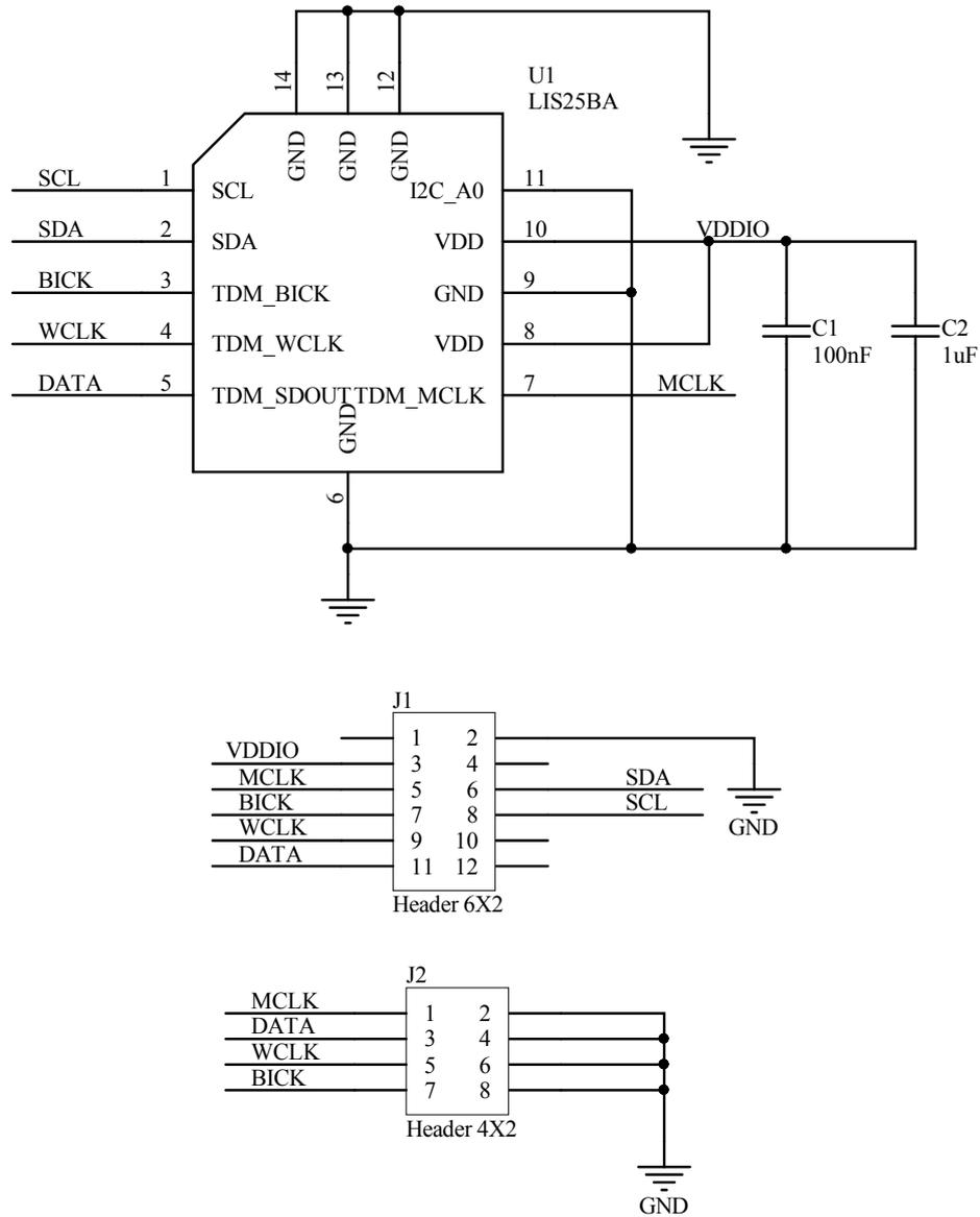
Figure 2. STEVAL-MKIGIBV3 circuit schematic
