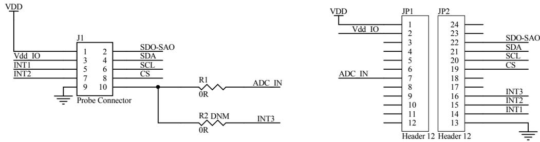
Figure 2. STEVAL-MKI200V1 board schematic
