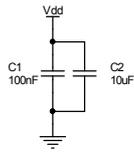
Figure 1. STEVAL-MKI186V1 circuit schematic
