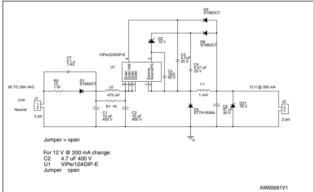
Figure 2. Circuit schematic for 16 V at 350 mA
