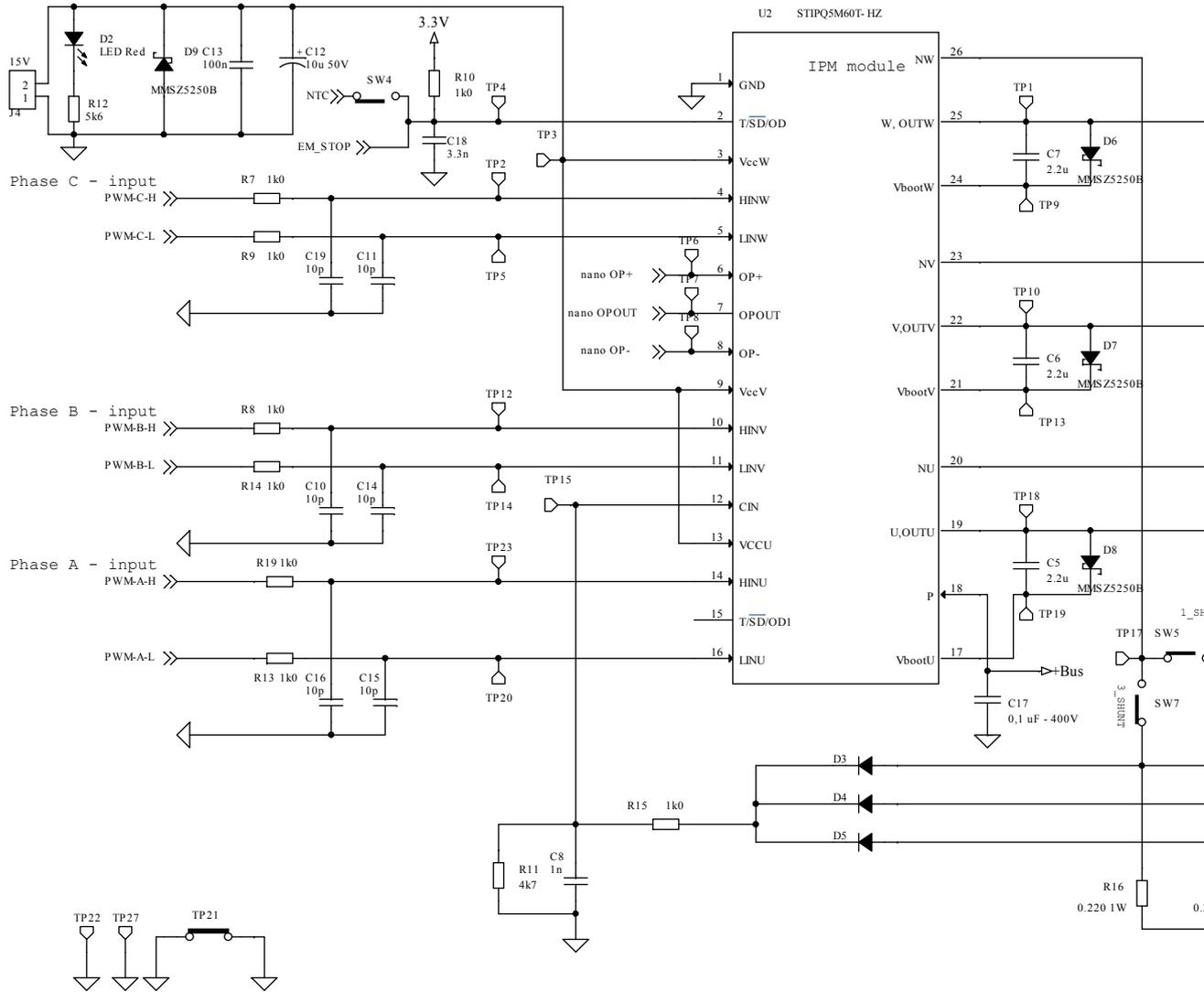
Figure 5. STEVAL-IPMNM5Q board schematic (5 of 5)
