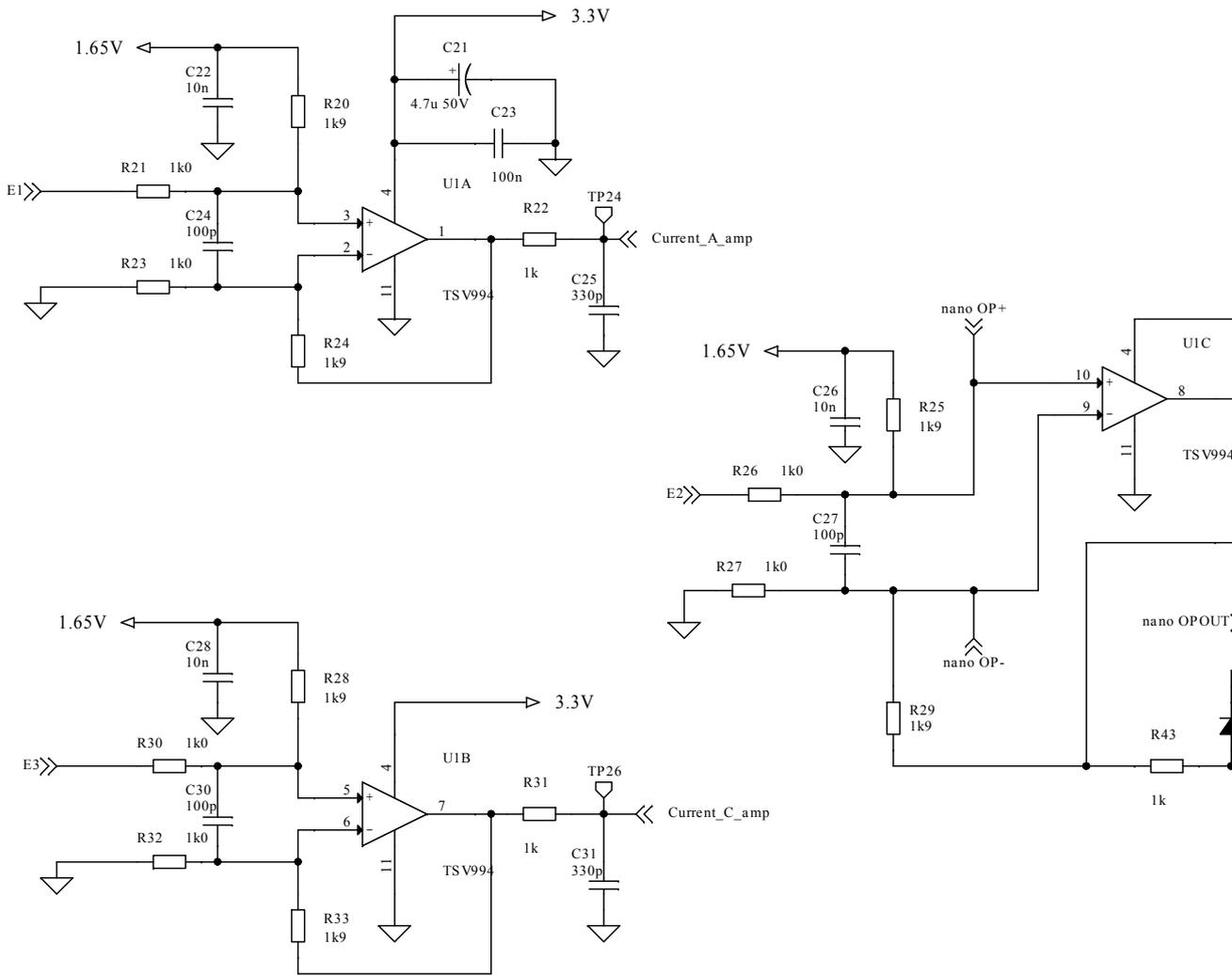
Figure 4. STEVAL-IPMNM5Q board schematic (4 of 5)
