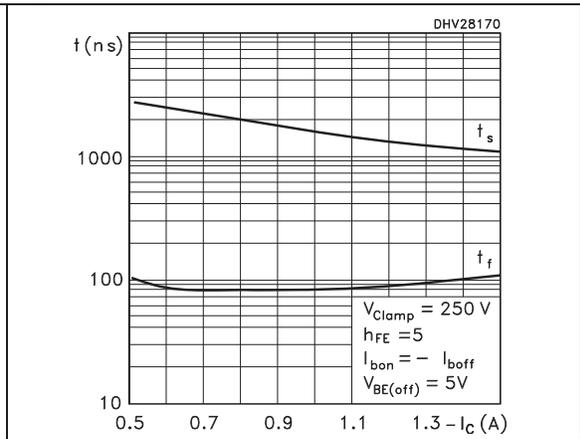
Figure 13. Resistive load storage time NPN
