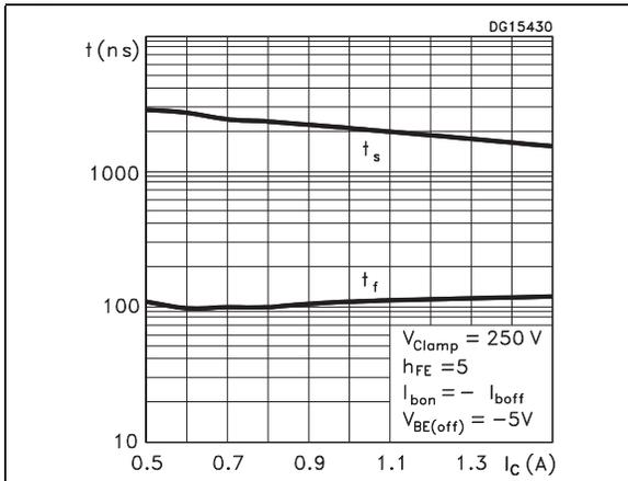
Figure 12. Resistive load fall time PNP
