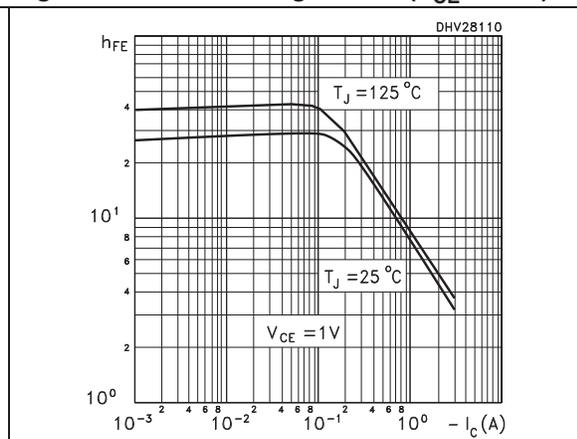
Figure 4. DC current gain NPN ( $V_{CE} = 1\text{ V}$ )
