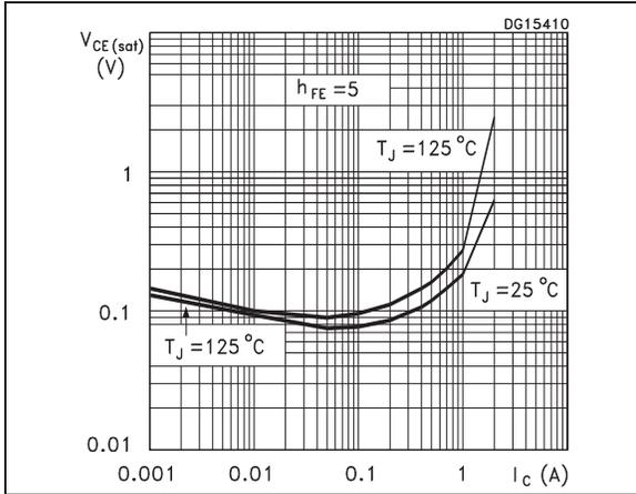
Figure 8. Collector emitter saturation voltage PNP
