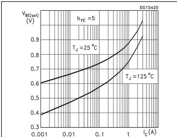
Figure 10. Base emitter saturation voltage PNP
