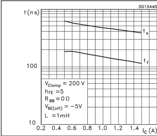
Figure 14. Resistive load storage time PNP
