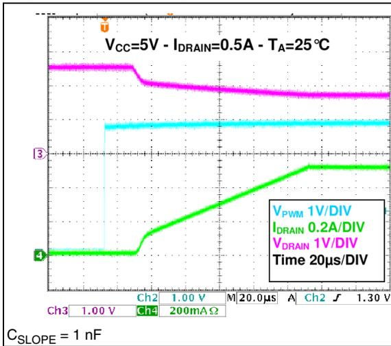
Figure 14. Dimming operation: Fall
