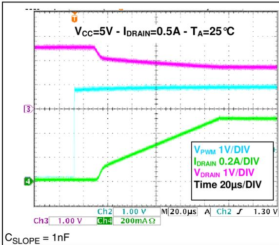
Figure 14. Dimming operation: Fall
