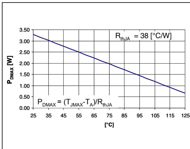
**Figure 17. Maximum power dissipation vs  $T_A$  for PowerSO-8**
