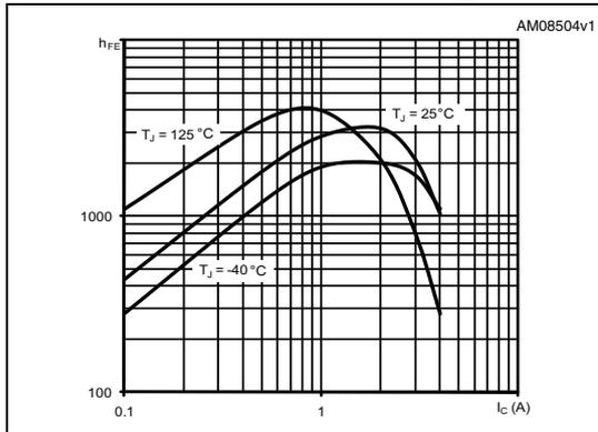
**Figure 5. DC current gain ( $V_{CE} = 5\text{ V}$ )**
