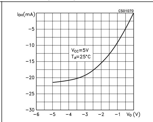
Figure 12. Driver output current vs. output low voltage
