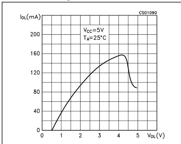
Figure 13. Driver output current vs. output high voltage
