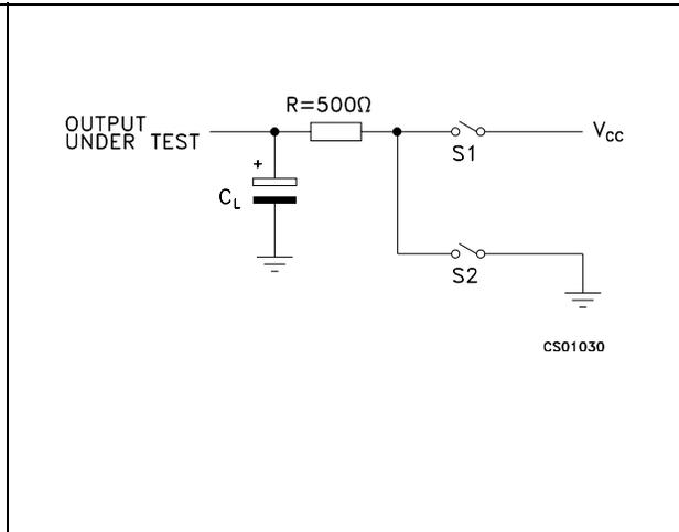
Figure 6. Driver propagation delay
