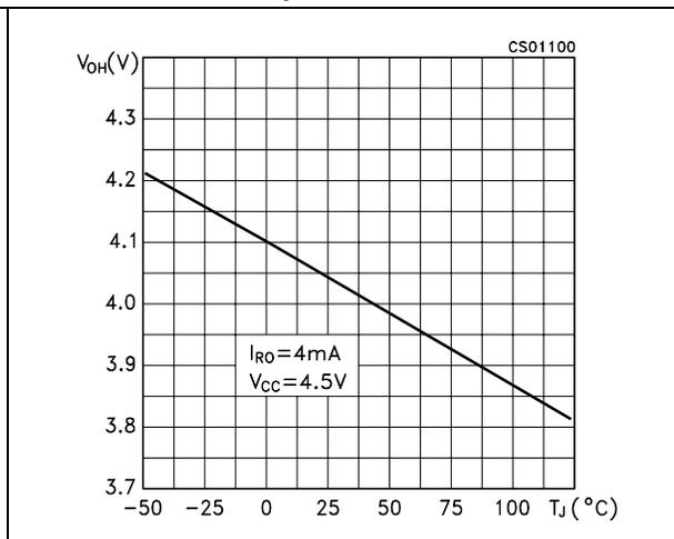
**Figure 16. Receiver low level output voltage vs. temperature**
