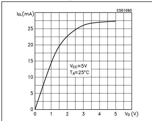
Figure 11. Receiver output current vs. output high voltage
